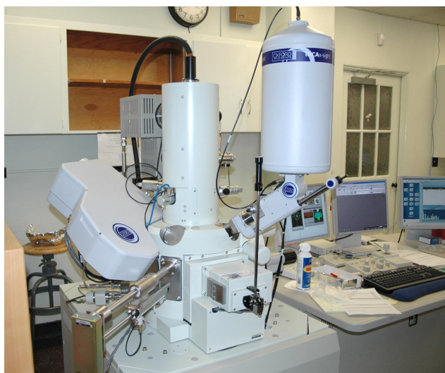
Figure 3.2.2.2.3.1. JEOL 7000F FEG-SEM with EBSD, EDS and WDS detectors.
