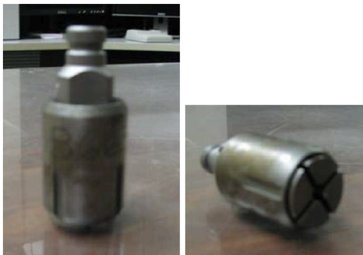
Figure 2.1.4. Type D end fittings that are attached to the end of each fuel rod for handling.
