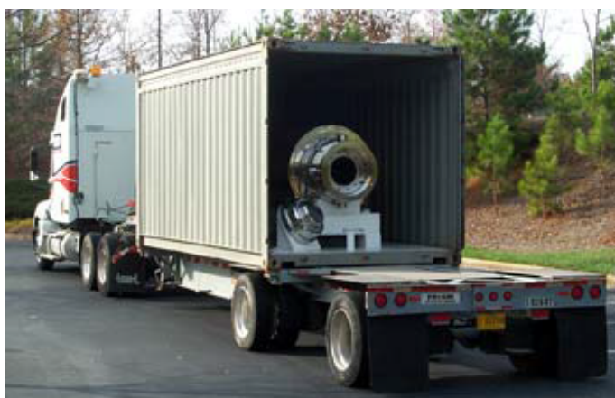
Figure 2.1.1. NAC-LWT loaded in an ISO-container on a transport trailer demonstrating the transport configuration. The lid is not installed in this image, nor is the end-wall of the ISO-container.
