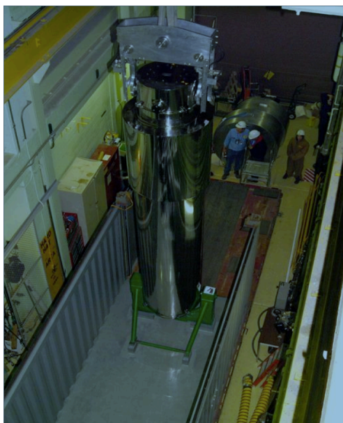
Figure 2.1.2. A NAC-LWT cask being unloaded in HFEF. The cask is lifted out of the ISO-container and lowered into the cask transfer tunnel and onto the cask transfer cart.
