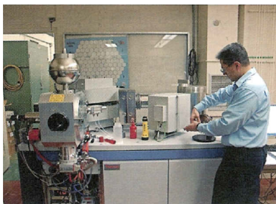
Figure 3.2.2.3.1. Finnigan MAT 262 Thermal Ionization Mass Spectrometer
