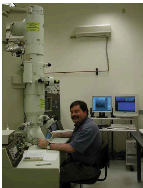
Figure 3.2.2.2.3.2. JEOL 2010F scanning transmission electron microscope
