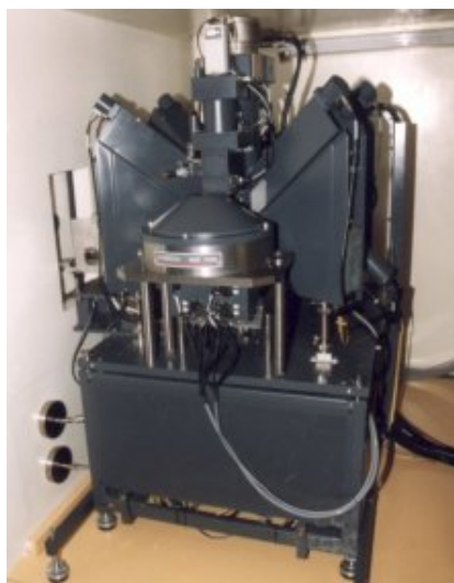
Figure 3.2.2.4.1. CAMECA SX100-R shielded electron probe micro analyzer.
