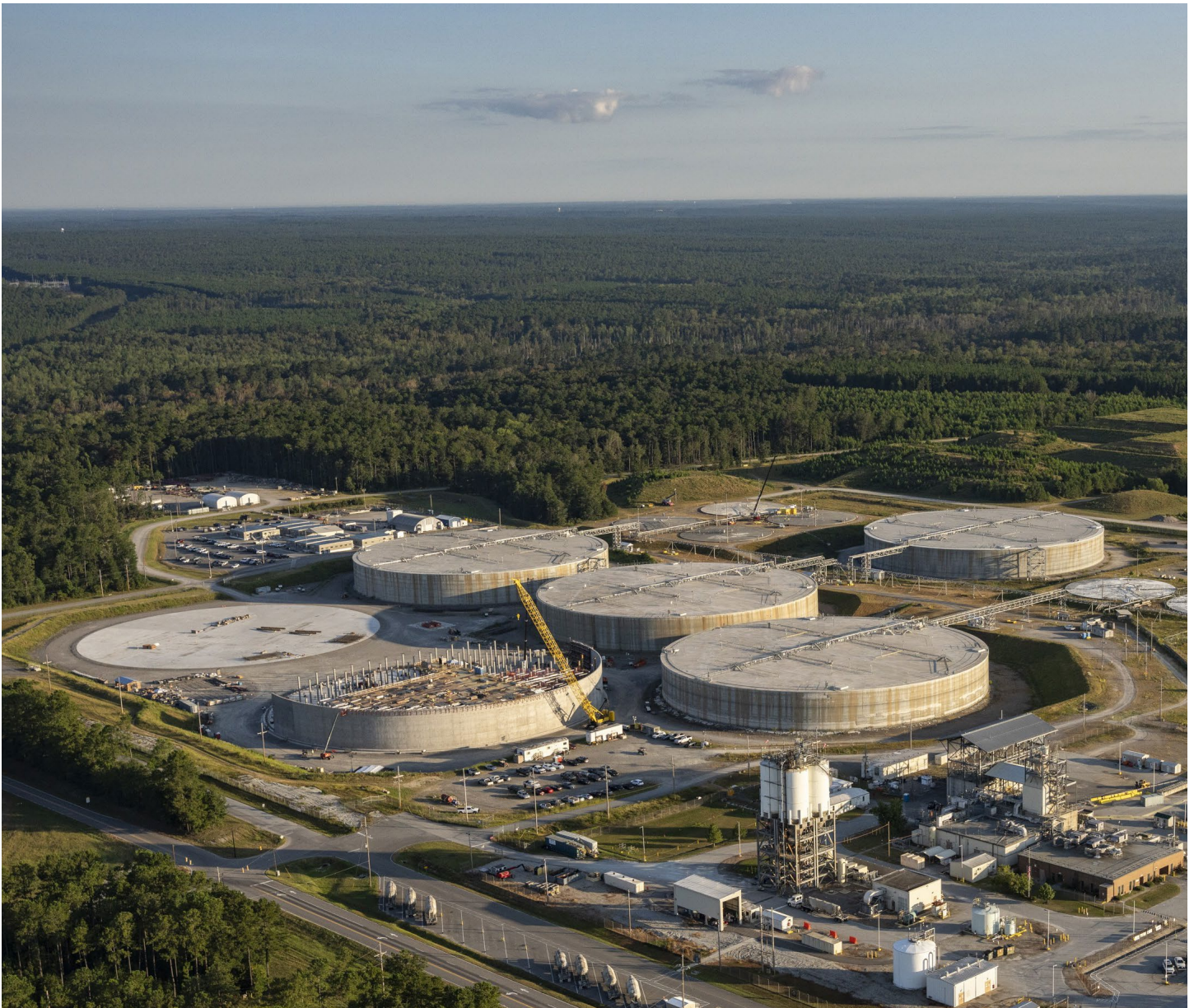
Saltstone Disposal Units are permanent disposal units of the saltstone grout at the Savannah River Site. The smaller SDUs can be seen in the background and right portion of the photo among the landscape of the mega-volume disposal units.
