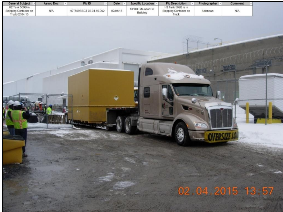
Figure 22. Shipping Tank 509A in custom oversize container
