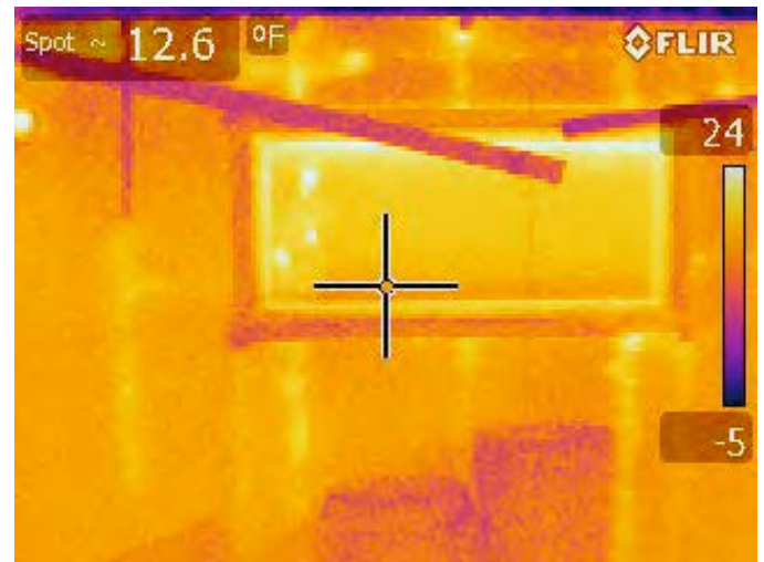
Glen Joe Sr. Home. Exterior view. Thermal imaging shows heat leakage both at windows and along studs.
