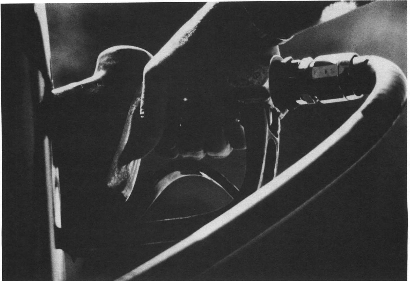
*Gasoline pump nozzles such as this 1981 style were replaced at many gasoline service stations after most Northeastern States mandated the use of anti-vapor gasoline pump nozzles in the late 1980's. Hydrocarbon emissions during refueling had increased as more butane and benzene were added to motor gasoline to replace lead.*
