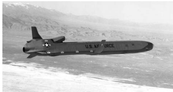
W80 warhead and its delivery system, the Air Launched Cruise Missile
