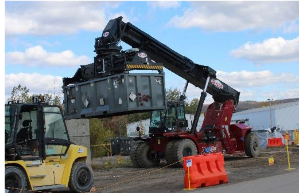
A reach-stacker removes a full waste container from the demolition area
