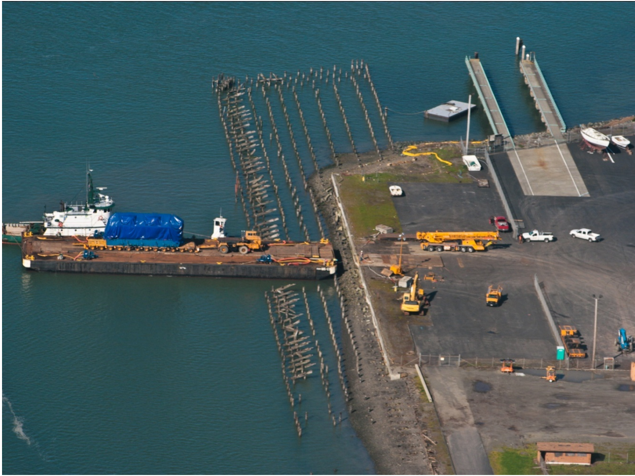
Figure 4-38. Barge with Wartsila Engine Arriving at Fields Landing Terminal
