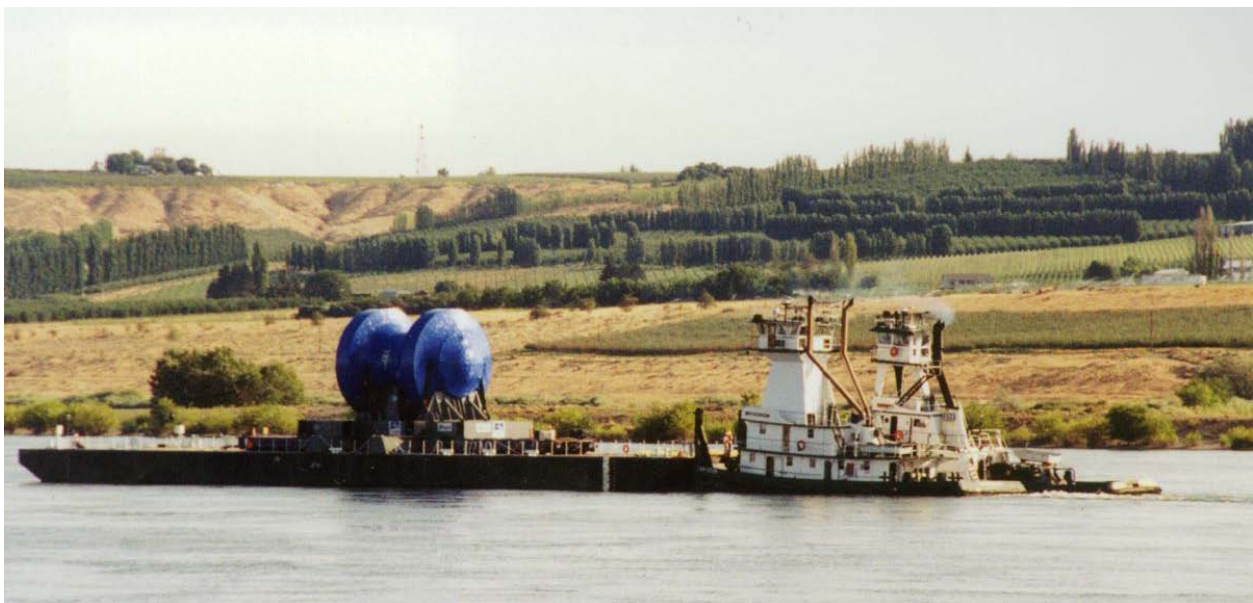
Figure 4-30. Trojan Reactor Pressure Vessel Being Transported by Barge
