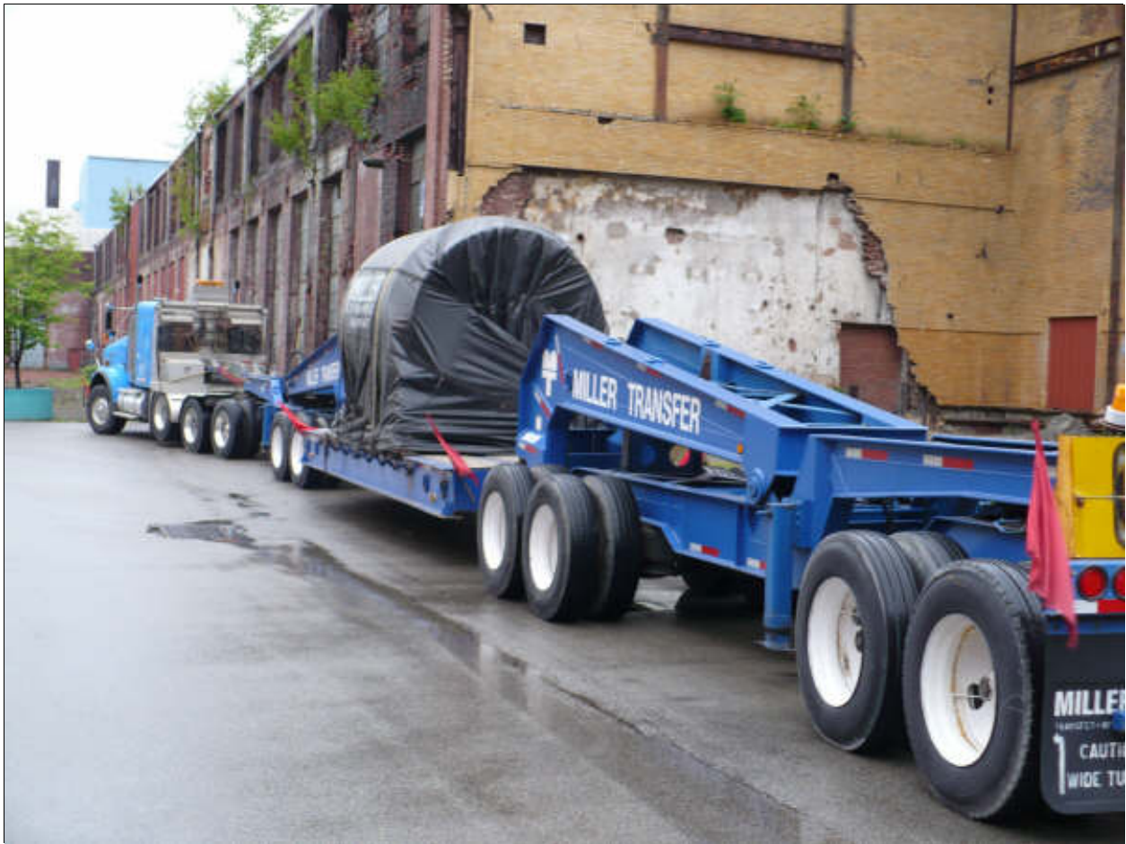
Figure 4-7. HI-STAR HB Cask Transported by Heavy Haul Truck
