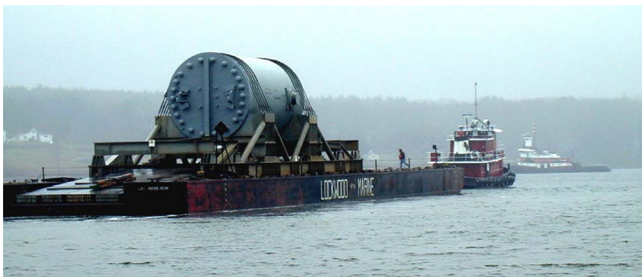
Figure 4-25. Maine Yankee Reactor Pressure Vessel Being Transported on Barge
