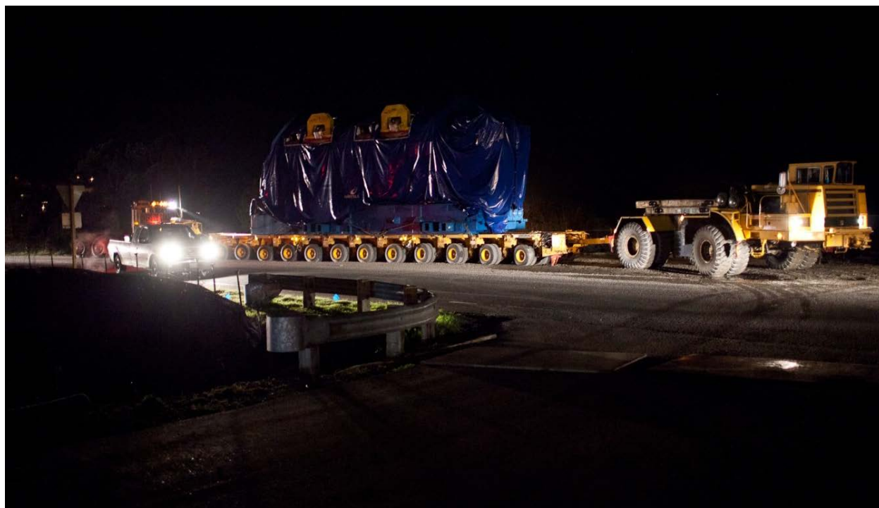
Figure 4-40. Wartsila Engine Being Transported by Heavy Haul Truck to Humboldt Bay Generating Station
