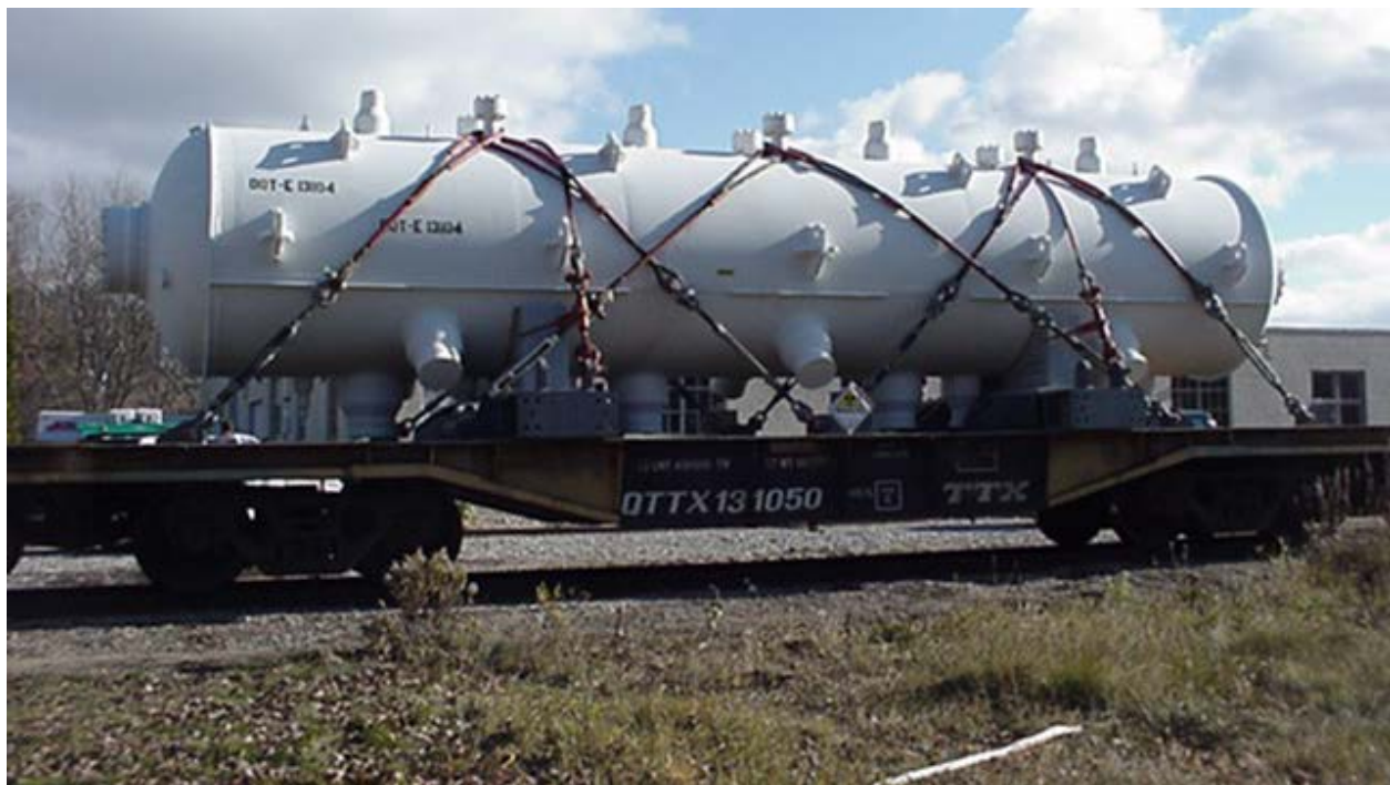
Figure 4-18. Big Rock Point Steam Drum on Railcar
