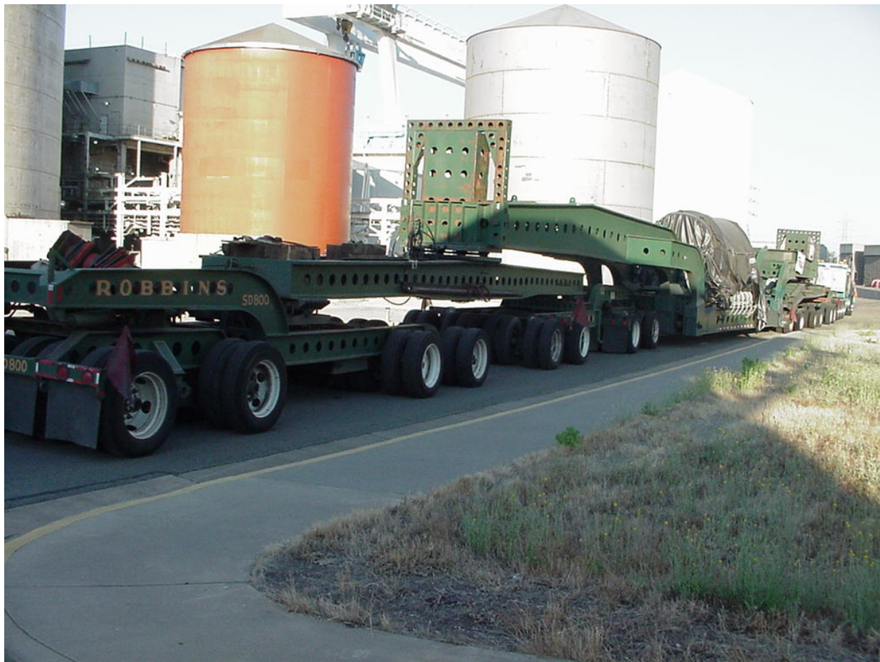
Figure 4-6. MP187 Cask Transported by Heavy Haul Truck
