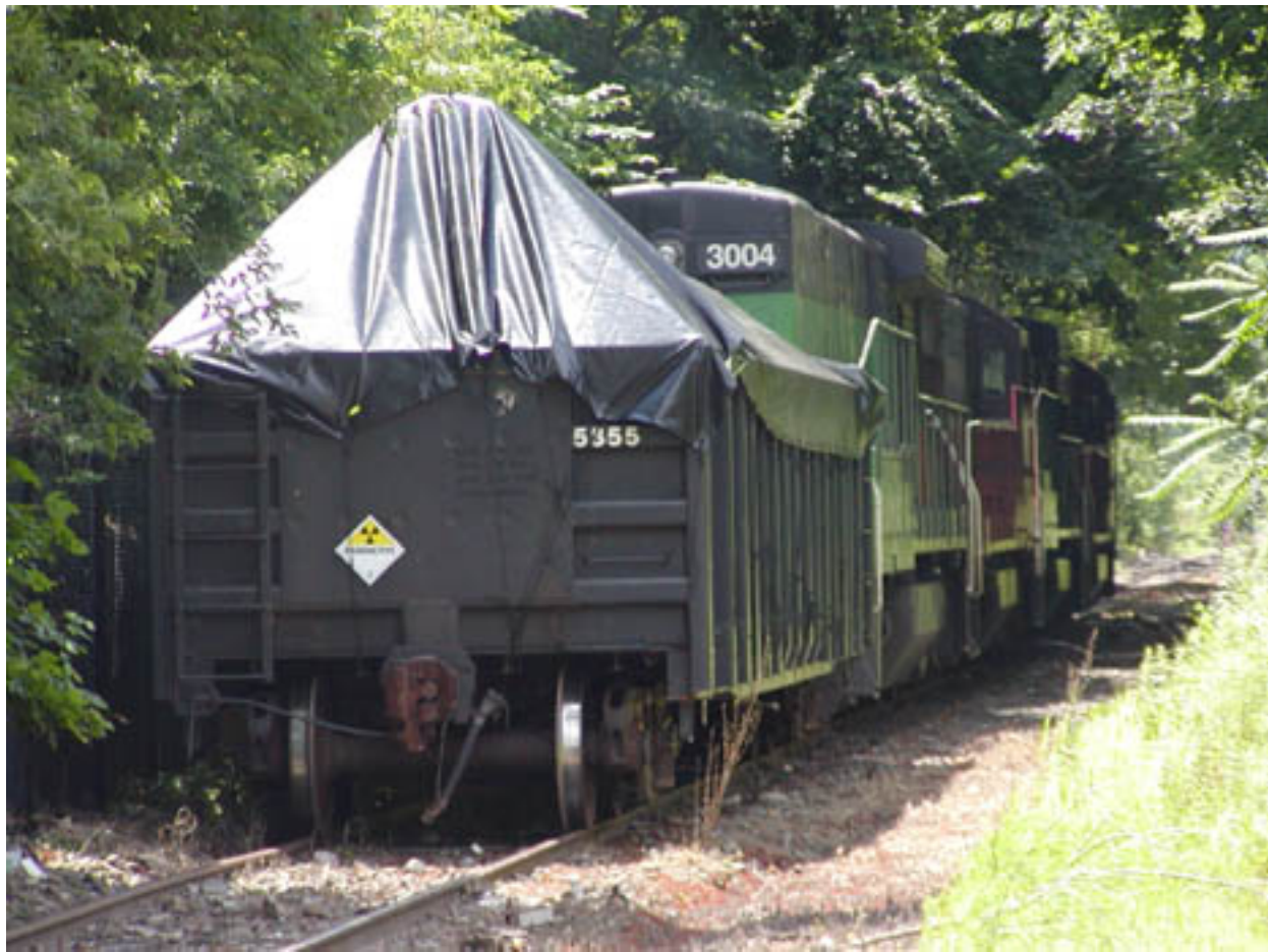
Figure 4-21. Connecticut Yankee Pressurizer at Portland Railhead
