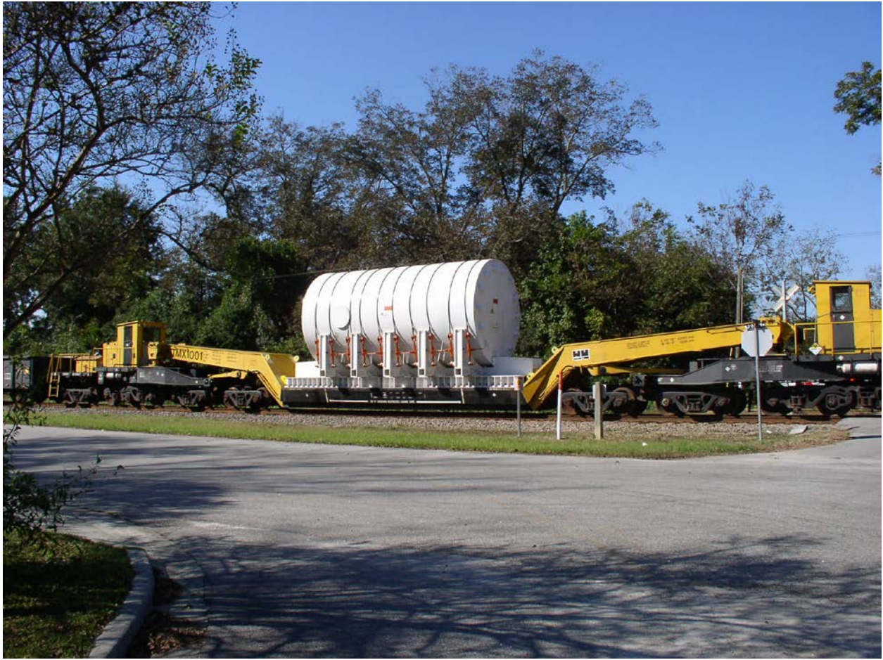
Figure 4-15. Big Rock Point Reactor Pressure Vessel on Railcar
