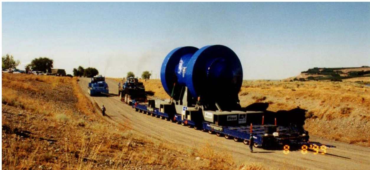
Figure 4-32. Trojan Reactor Pressure Vessel Being Transported by Heavy Haul Truck
