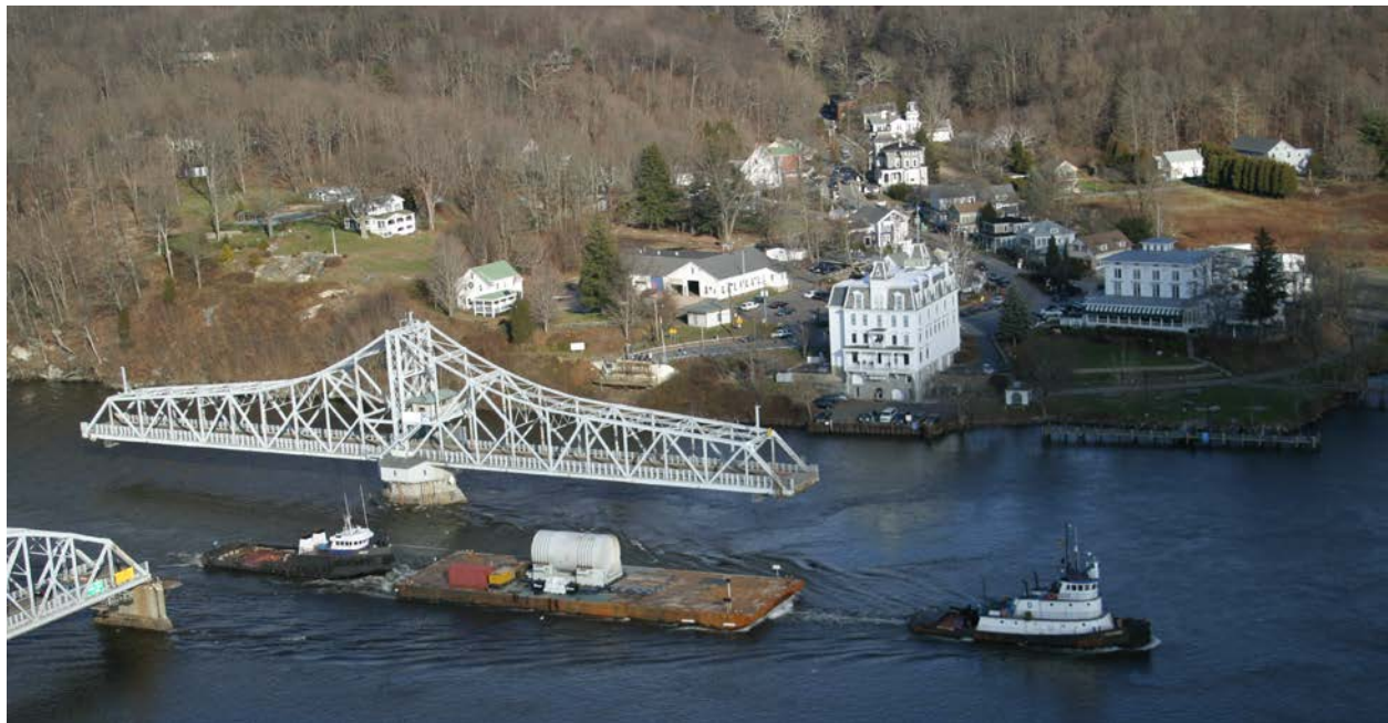
Figure 4-28. Connecticut Yankee Reactor Pressure Vessel Being Transported on Barge in the Connecticut River
