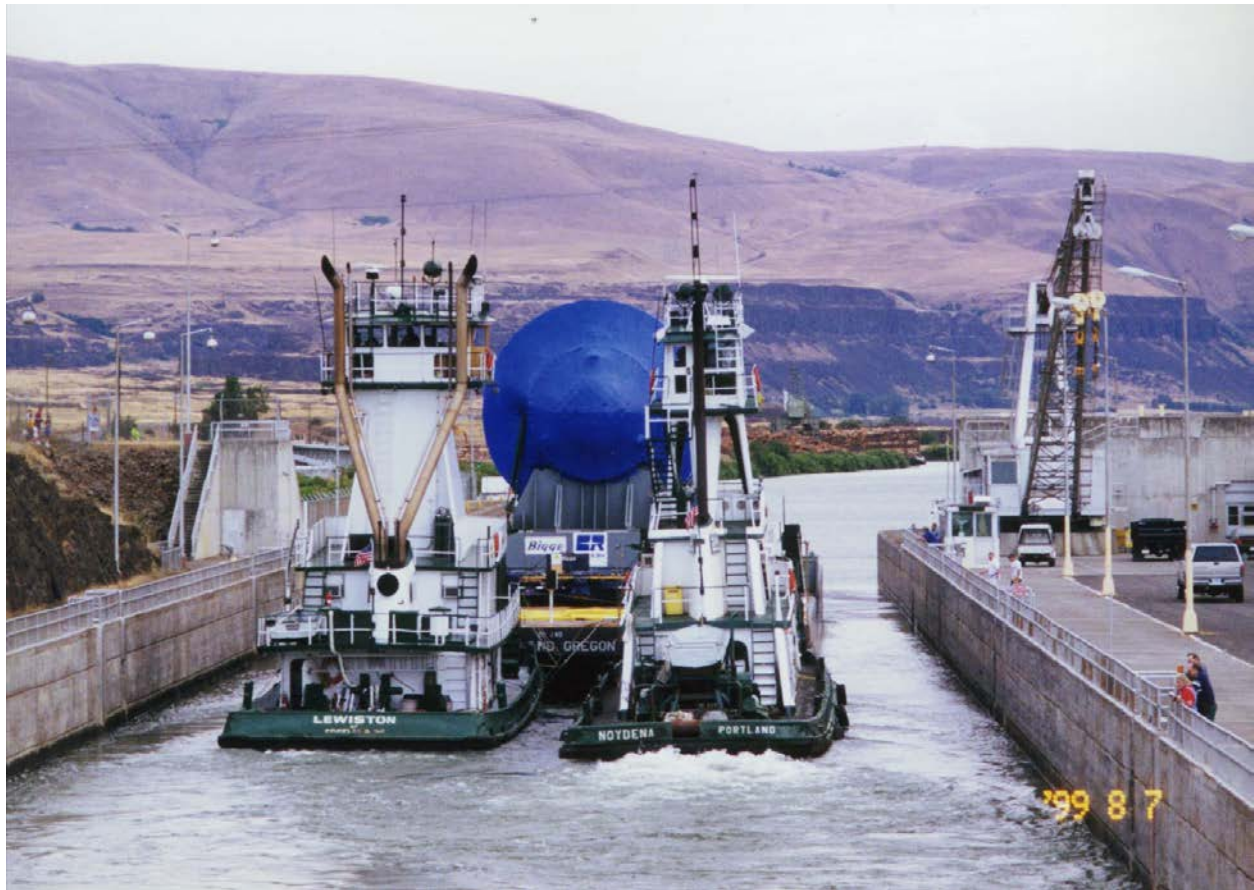
Figure 4-31. Trojan Reactor Pressure Vessel Passing Through Locks on the Columbia River
