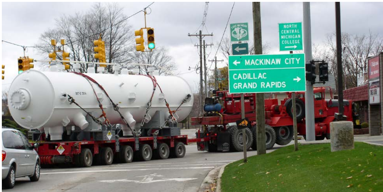
Figure 4-17. Big Rock Point Steam Drum on Heavy Haul Truck
