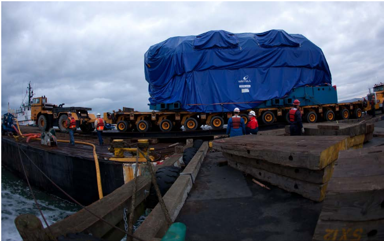
Figure 4-36. Wartsila Engine Being Loaded on a Barge
