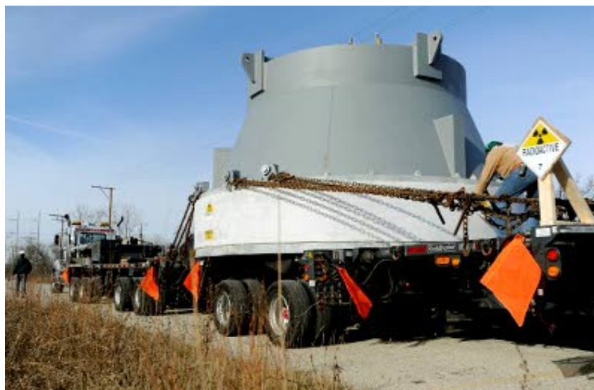
Figure 4-23. Zion Reactor Head on Heavy Haul Truck Transporter
