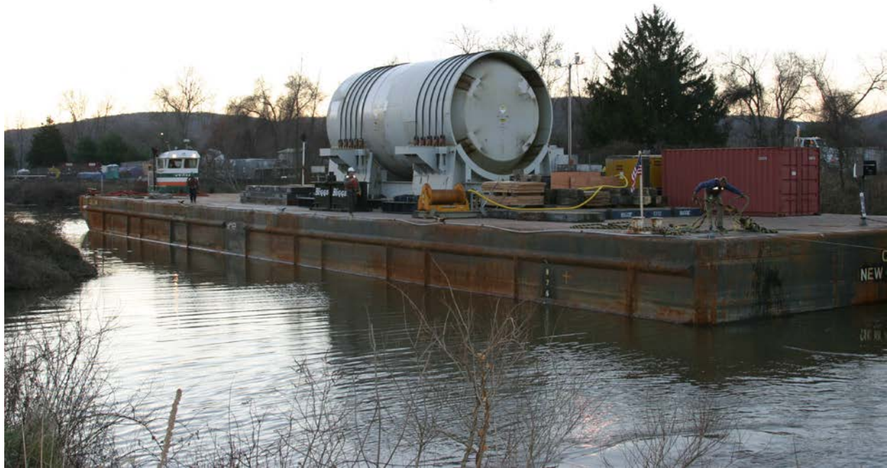
Figure 4-27. Connecticut Yankee Reactor Pressure Vessel Being Transported on Barge
