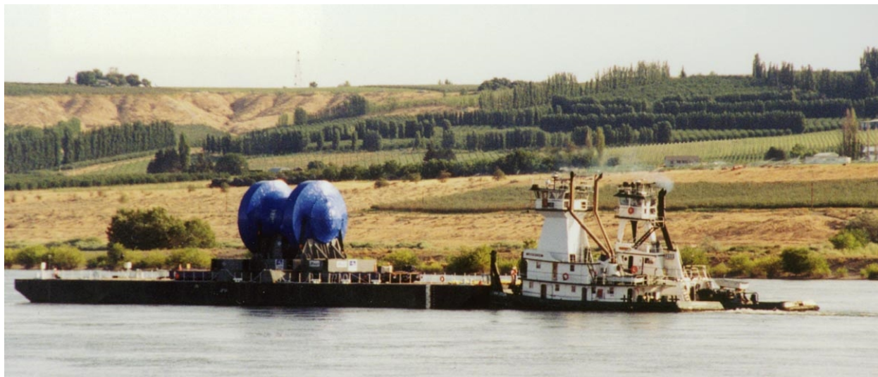
Figure 2-100. Trojan Reactor Pressure Vessel Being Transported by Barge
