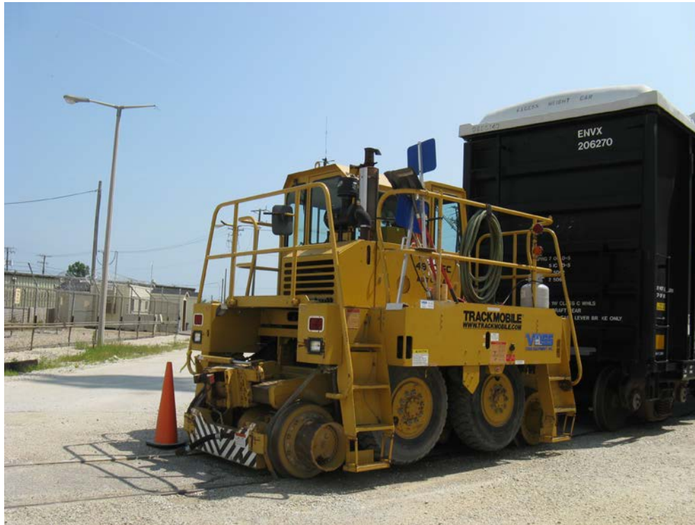
Figure 2-122. Trackmobile Used to Move Railcars On-site
