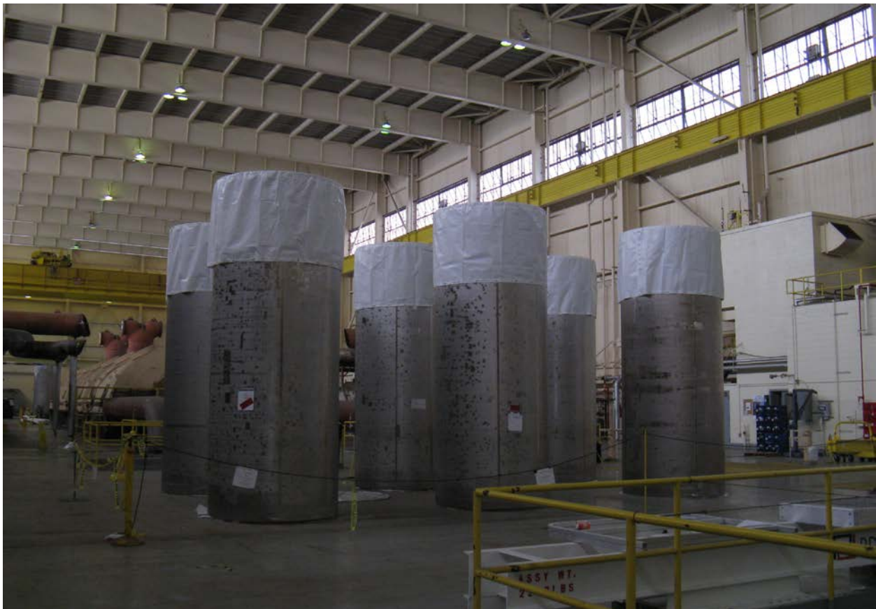
Figure 2-119. Empty Used Nuclear Fuel Transportable Storage Canisters at Zion
