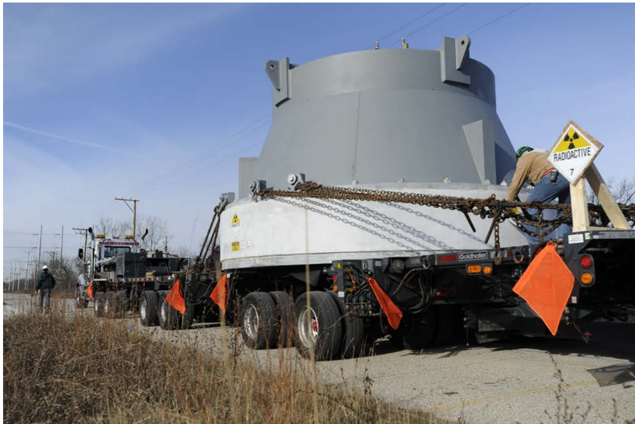
Figure 2-125. Zion Reactor Head on Heavy Haul Truck Transporter
