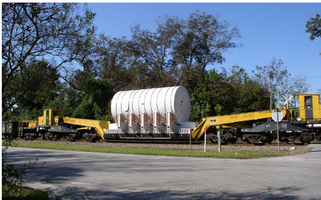
Figure 2-64. Big Rock Point Reactor Pressure Vessel on Railcar
