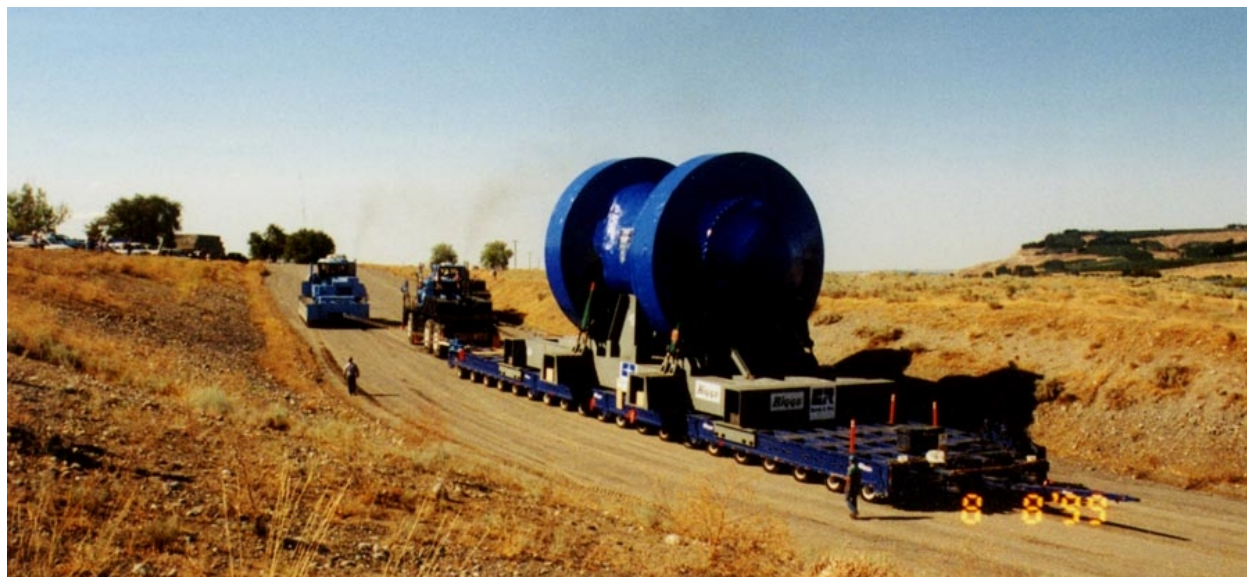
Figure 2-102. Trojan Reactor Pressure Vessel Being Transported by Heavy Haul Truck
