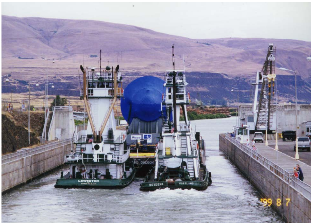
Figure 2-101. Trojan Reactor Pressure Vessel Passing Through Locks on the Columbia River
