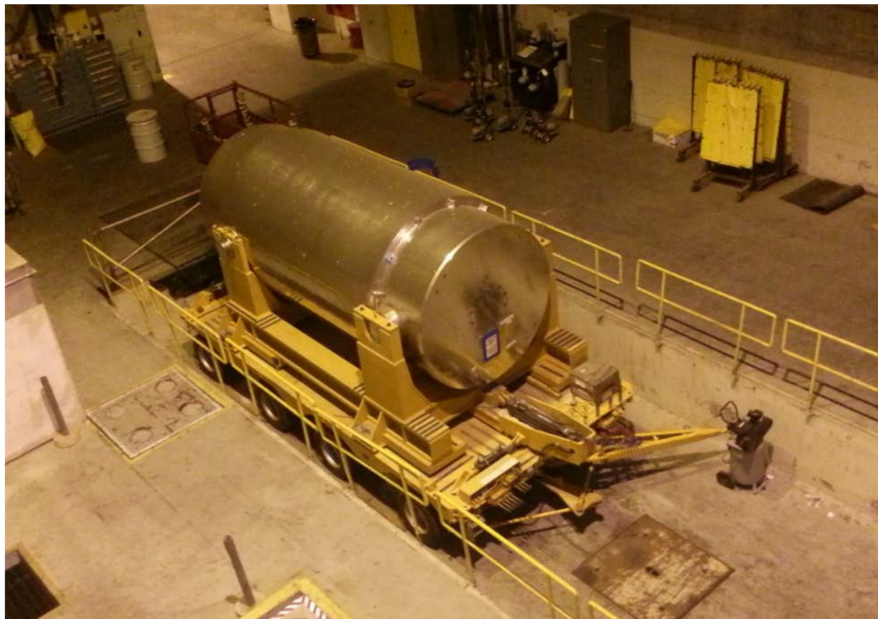
Figure 2-77. MP187 Transportation Cask at Rancho Seco
