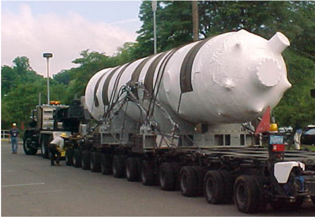
Figure 2-33. Connecticut Yankee Pressurizer on Heavy Haul Truck Transporter
