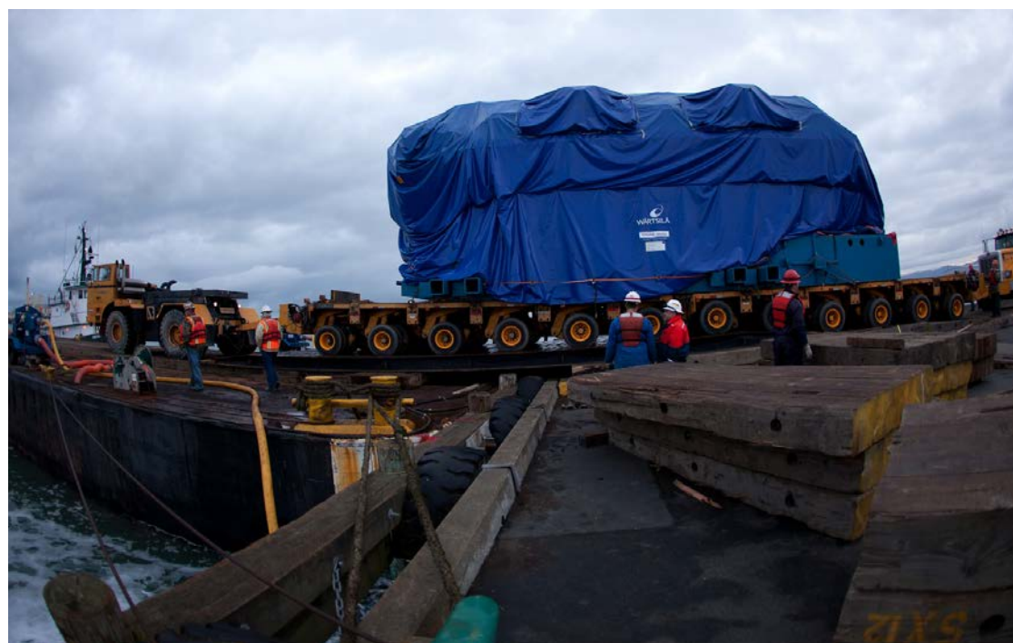
Figure 2-48. Wartsila Engine Being Loaded on a Barge
