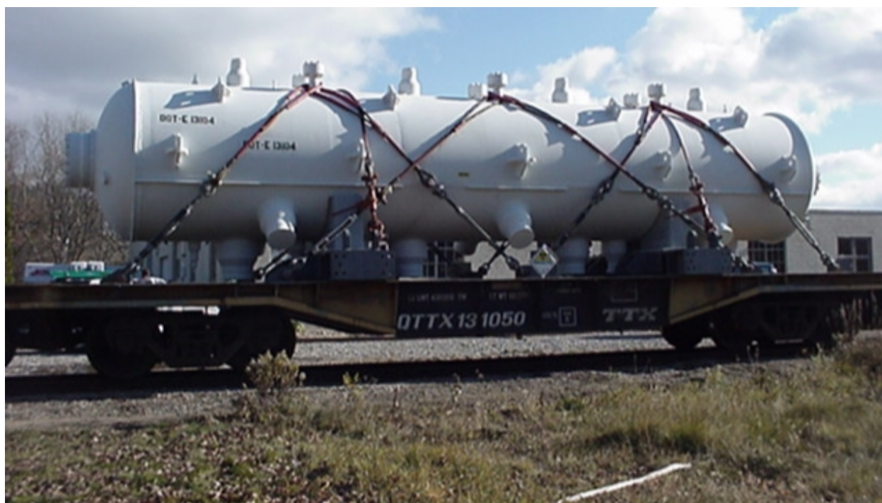
Figure 2-72. Big Rock Point Steam Drum on Railcar
