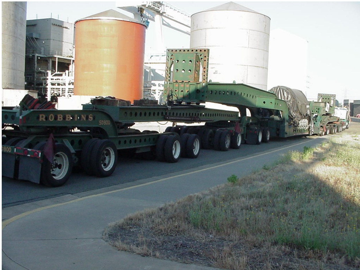
Figure 2-85. MP187 Cask Transported by Heavy Haul Truck
