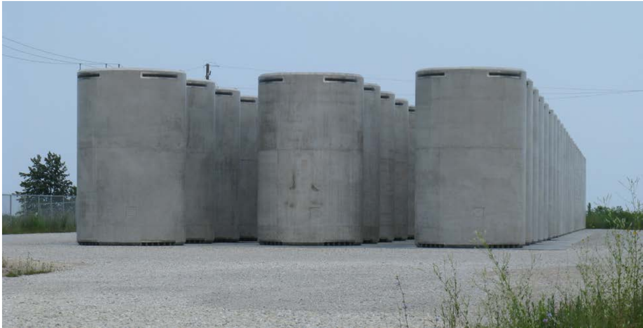
Figure 2-118. Vertical Concrete Storage Casks Staged at Zion
