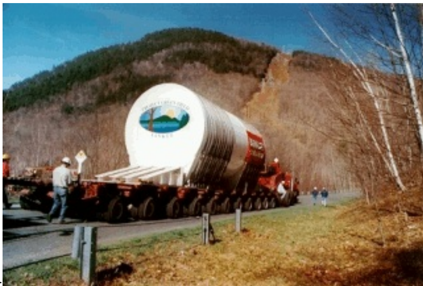
Figure 2-22. Yankee Rowe Reactor Pressure Vessel Being Transported by Heavy Haul Truck
