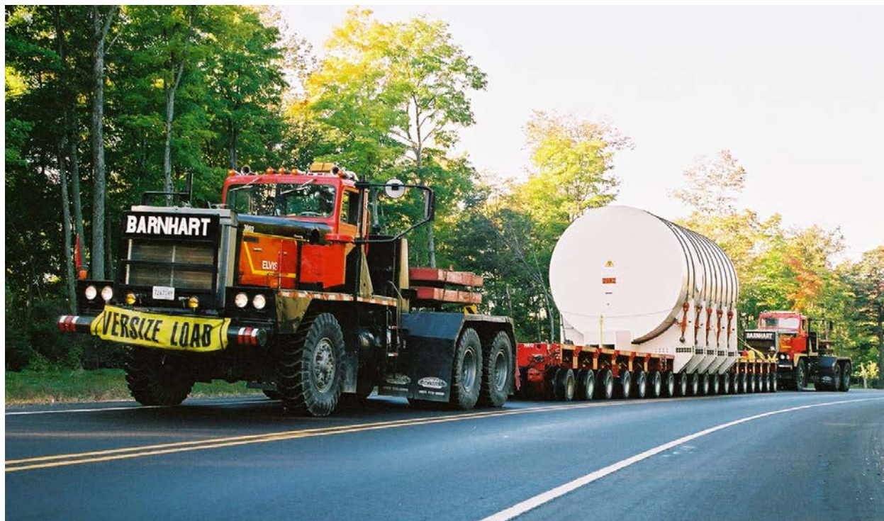
Figure 2-63. Big Rock Point Reactor Pressure Vessel on Heavy Haul Truck
