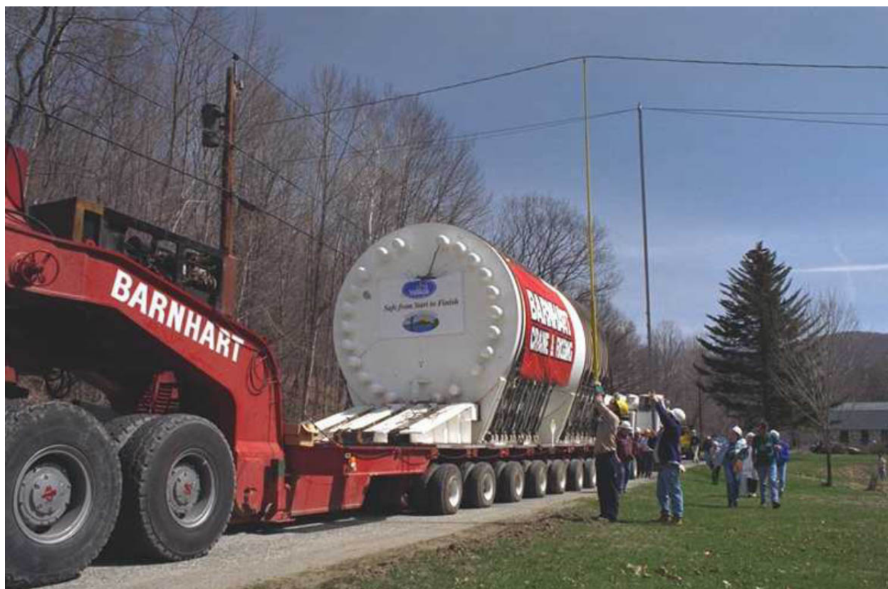
Figure 2-23. Yankee Rowe Reactor Pressure Vessel on Heavy Haul Truck Moving Under Power Lines
