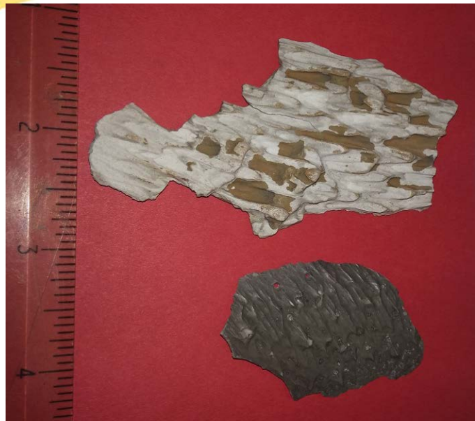
Wall scale, or “bark” formation indicates inconsistent conversion of the simulated waste.
