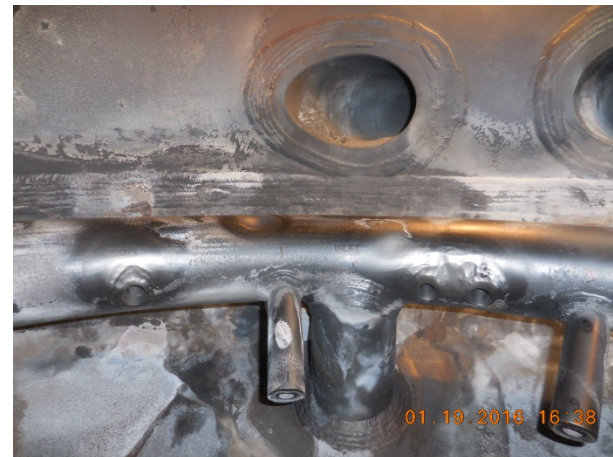
The ring header will have to be replaced because of erosion impacts.
