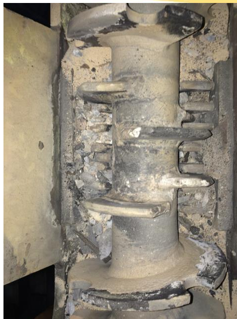
Cement-like materials damaged the auger-grinder.
