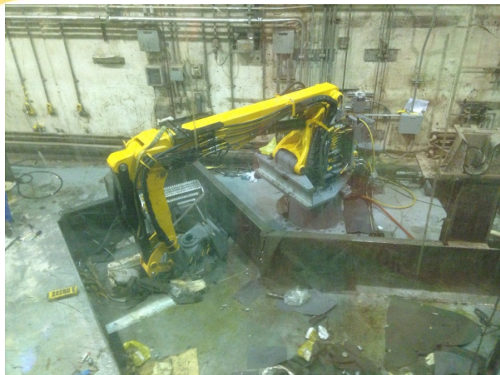
Above: New Brokk 400 installed in South Box Line
