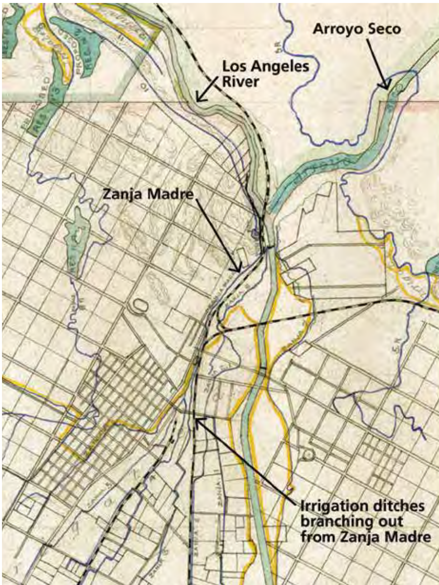
The Los Angeles River provided the original water source for El Pueblo and then the City of Los Angeles. The Zanja Madre, or “Mother Ditch”, conveyed water from the river to El Pueblo. The photo, dated 1862, shows the water wheel which lifted water from the river into the Zanja Madre. The Zanja Madre conveyed water into a network of other irrigation ditches that were developed over time as shown in the map (ca. 1880s). Portions of the Zanja are still being unearthed today. Photo: Security Pacific National Bank Collection/Los Angeles Public Library. Map: Detail Irrigation Map Southern California-Los Angeles ca.1880s, William Hammond Hall Papers, 91-07-04, 91-06-10/California State Archives.
