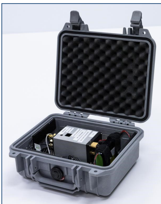
The Transport Security Tracking and Reporting (T-STAR) system is a DNN-developed technology that helps keep radiological material secure while in transit.
