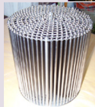
LEU core inserted into the Chinese MNSR at the CIAE.
