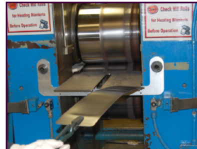
Example of a high-density LEU fuel being rolled.
