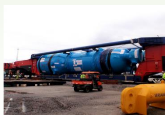
Completed Unit 2 steam generator arrives by rail and heavy lift of CA05 module (Courtesy of SCANA)
