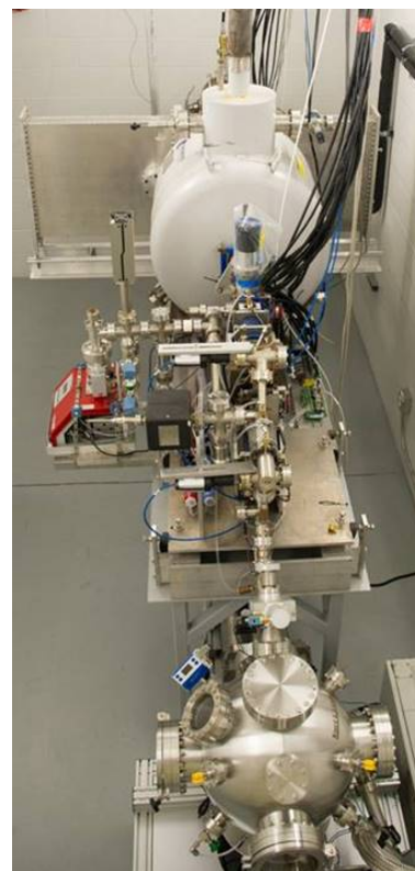
Figure 1. EBEAM system for additive manufacturing of SMR components housed at Mainstream Engineering Corp. in Rockledge, FL. Electron beam energies exceed 20\times higher than any other AM system.
