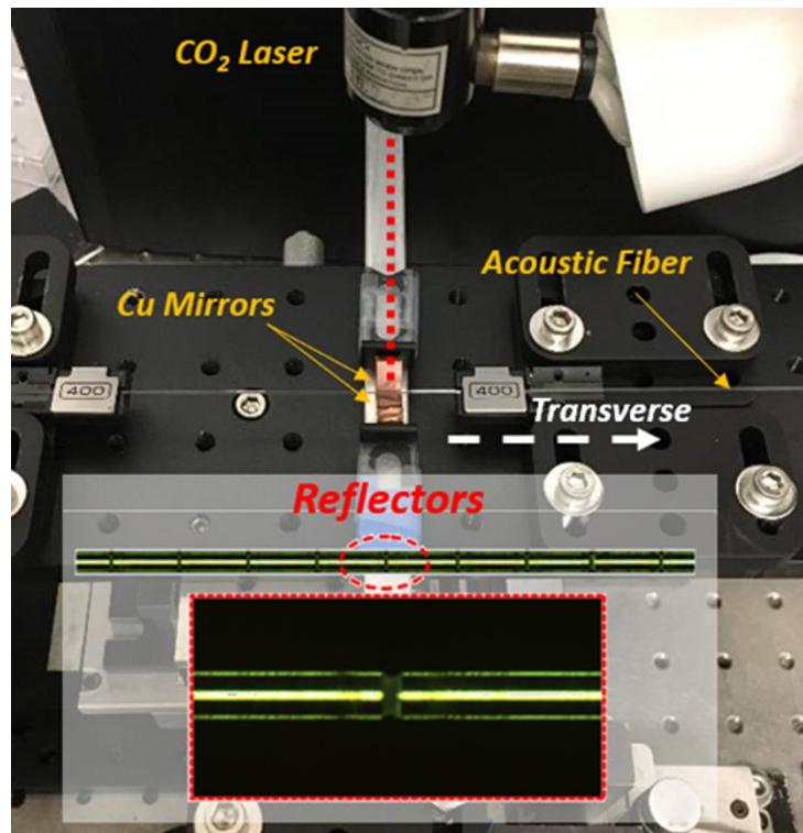
M3CA-17-VA-VT-0702-048 Reflector Element Fabrication and Testing (on schedule, 03/31/2019)
