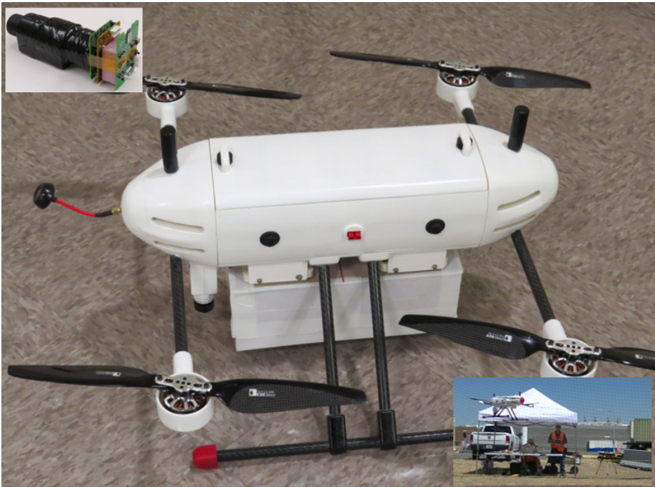
Figure E- 13. PNNL "Boxbotix" 3-D printed drone with insulated radiation detection sensor payload (top left inset image)
