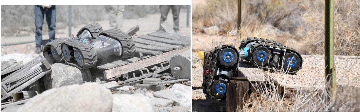
Figure A- 6. GAMMA actively articulated, dual-body, highly mobile platform
