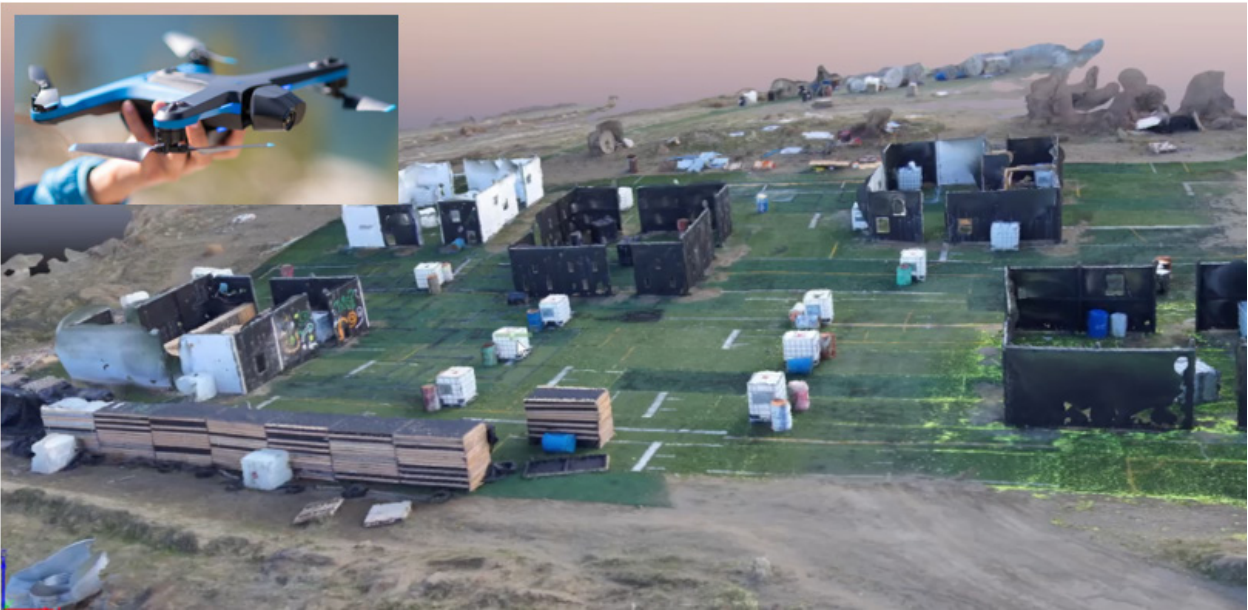
Figure E- 9. 3D photogrammetry video of a paint ball course generated by the PNNL "Skydio S2" drone
