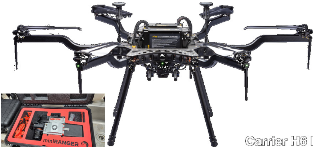
Figure E- 12. PNNL "Harris Carrier H6 Electric" UAS is equipped with the "Phoenix miniRanger" LIDAR and Camera system. The H6 will lift a 17.6 pound (8 kg) payload and will fly for 48 minutes when empty.
