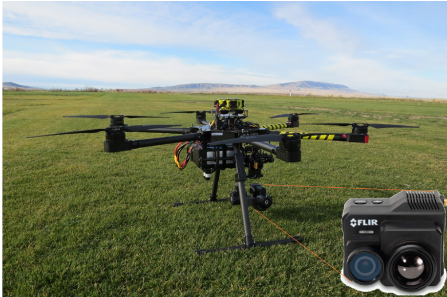
Figure E- 10. PNNL flies the FLIR 30Hz “Duo Pro R” - Electro Optic / Infrared camera mounted on a “Gremysy S1” gimbal system on the “X-6” multirotor UAS
