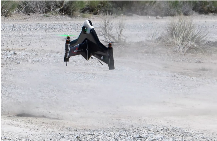
Figure E- 1. PNNL UAS capable of transitioning from VTOL to horizontal fixed wing flight. This embodiment can transport samples from the field to locations where sample analysis can be conducted. Other payloads include ground sample collections and wide area radiation detection sensors.
