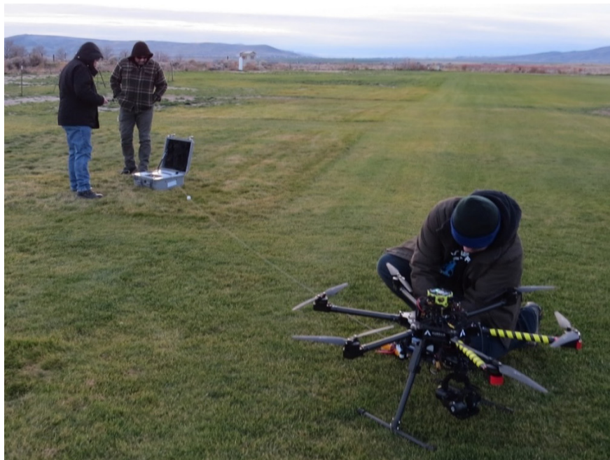
Figure E- 11. PNNL X-6 UAS attached to the “Blue Vigil” powered tether system. This allows the UAS to stay aloft indefinitely while powered by the ground-based power source
