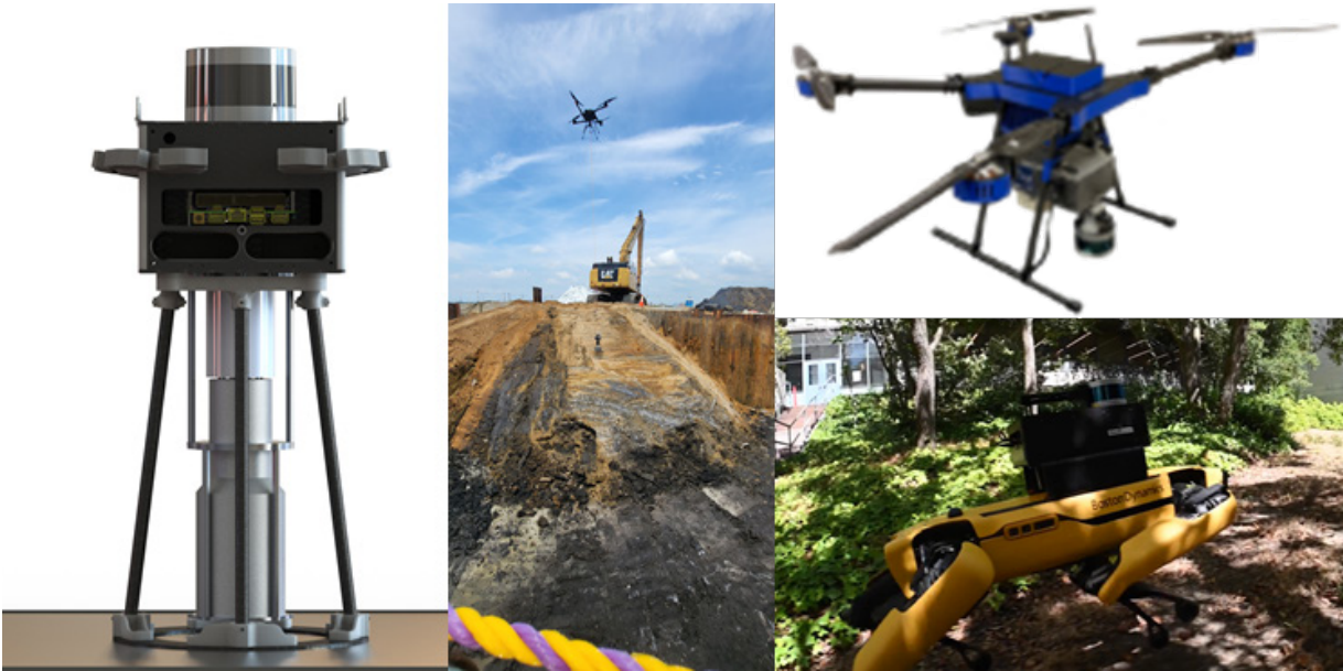
Figure F-1. Photographs of LAMP systems and uses on robotic platforms. (Left) Chandelier LAMP, a NaI(Tl) based gamma-ray detector designed to be slung below UAVs. (Left-center) Chandelier being carried by a UAV in a remediation excavation at the Deepwater FUSRAP site. (Top-right) The neutron and gamma-sensitive NG LAMP system mounted to a Theiss UAV. (Bottom-right) NG LAMP carried on a Boston Dynamics Spot quadruped robot.
