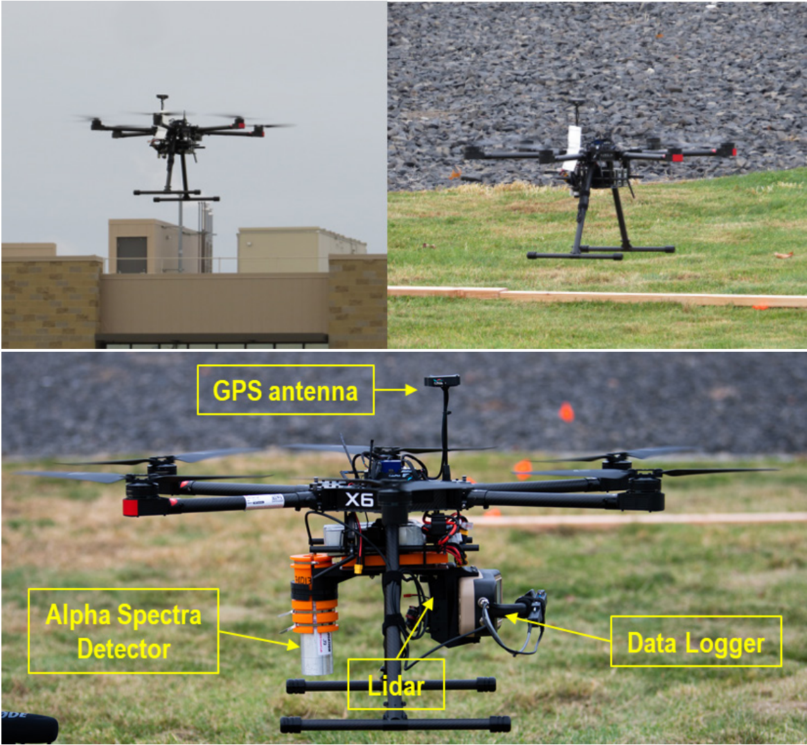
Figure E- 7. Above - PNNL "X-6" multirotor UAS exercises low altitude control and (below) carries a sodium iodide radiation detection sensor to survey sources on the ground
