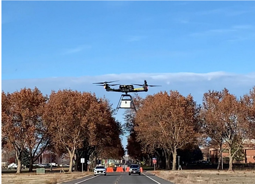
Figure E- 3. PNNL "Alta-X" quad copter capable of carrying 10 pounds of payload for over 30 minutes (or up to 35 pounds for about 11 minutes) is shown performing AI/ML augmented object recognition with onboard edge computing resources
