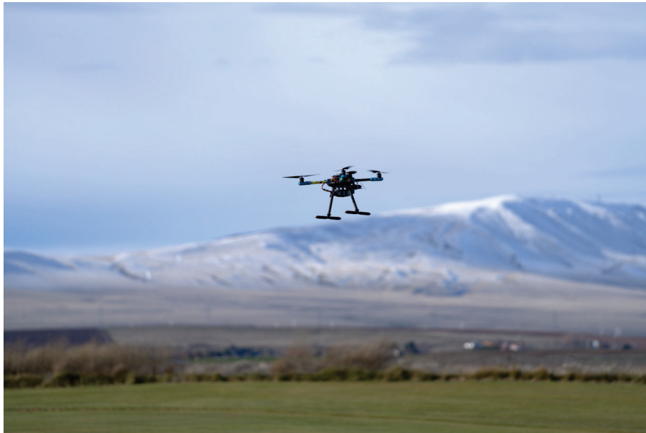
Figure E- 4. A PNNL training drone is flown by students to gain skills required to become PNNL Certified UAS Pilots. Pilots at PNNL are trained and certified by instructors on each airframe that they fly. The PNNL Remote and Autonomous Systems Lab operates several of these small drones and makes them available to projects with payloads under two pounds. PNNL has procedures that allow multiple drones to fly simultaneously in the same general airspace.
