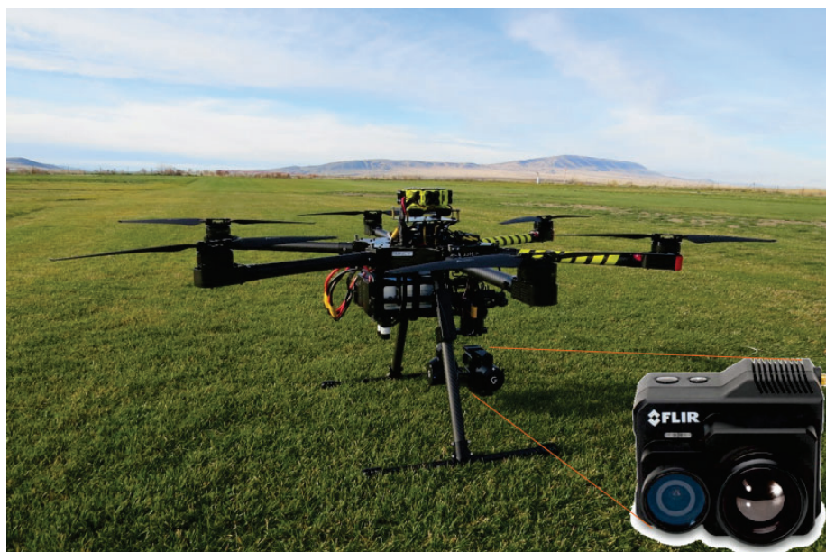
Figure E- 10. PNNL flies the FLIR 30Hz “Duo Pro R” - Electro Optic / Infrared camera mounted on a “Gremsy S1” gimbal system on the “X-6” multirotor UAS
