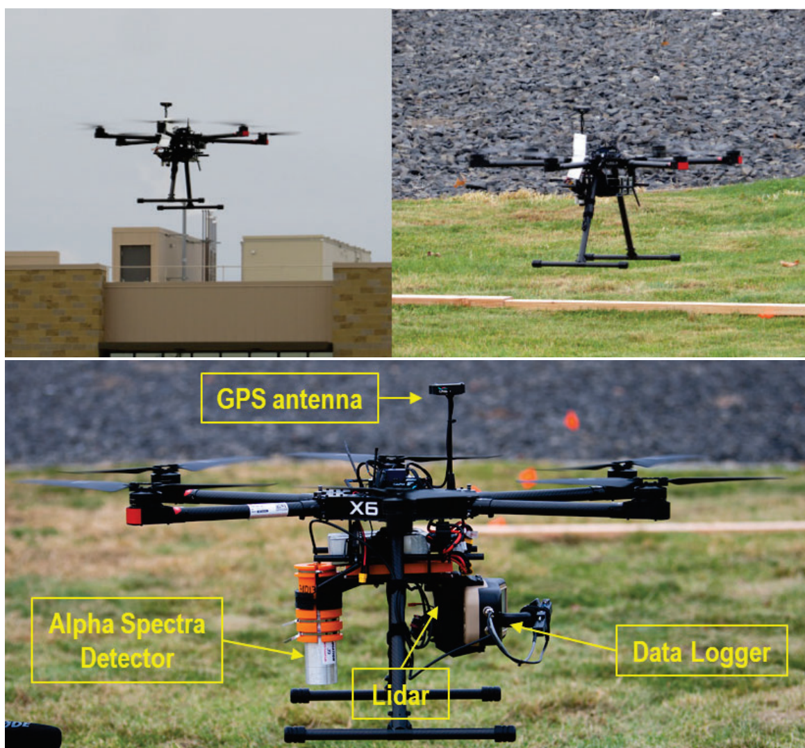
Figure E- 7. Above - PNNL "X-6" multirotor UAS exercises low altitude control and (below) carries a sodium iodide radiation detection sensor to survey sources on the ground
