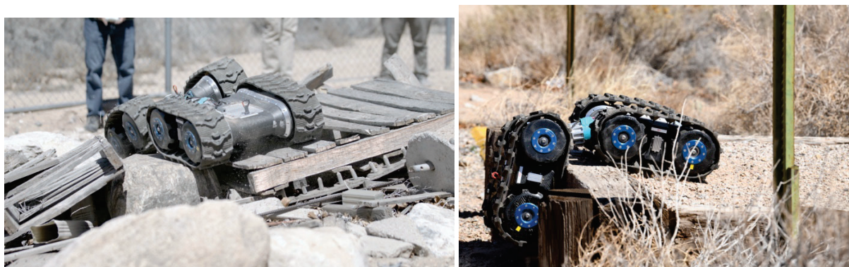
Figure A- 3. GAMMA actively articulated, dual-body, highly mobile platform
