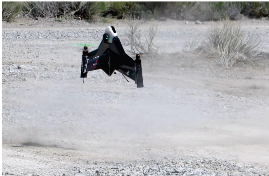
Figure E- 1. PNNL UAS capable of transitioning from VTOL to horizontal fixed wing flight. This embodiment can transport samples from the field to locations where sample analysis can be conducted. Other payloads include ground sample collections and wide area radiation detection sensors.
