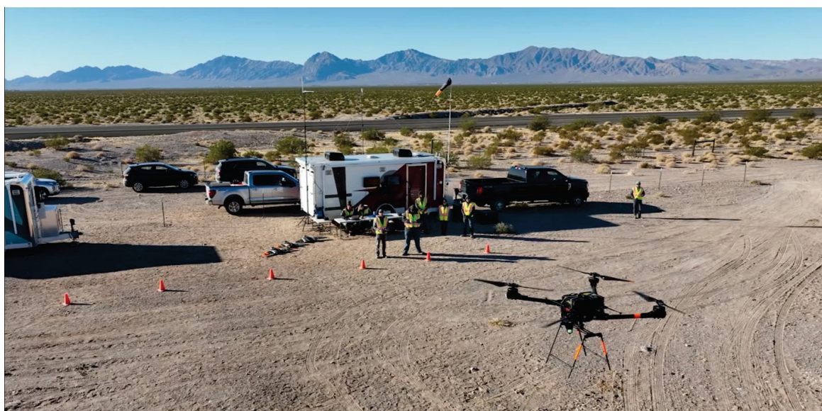
Figure A- 5. UAS Aerial Manipulation pulling a 10lb Pelican case while in flight
