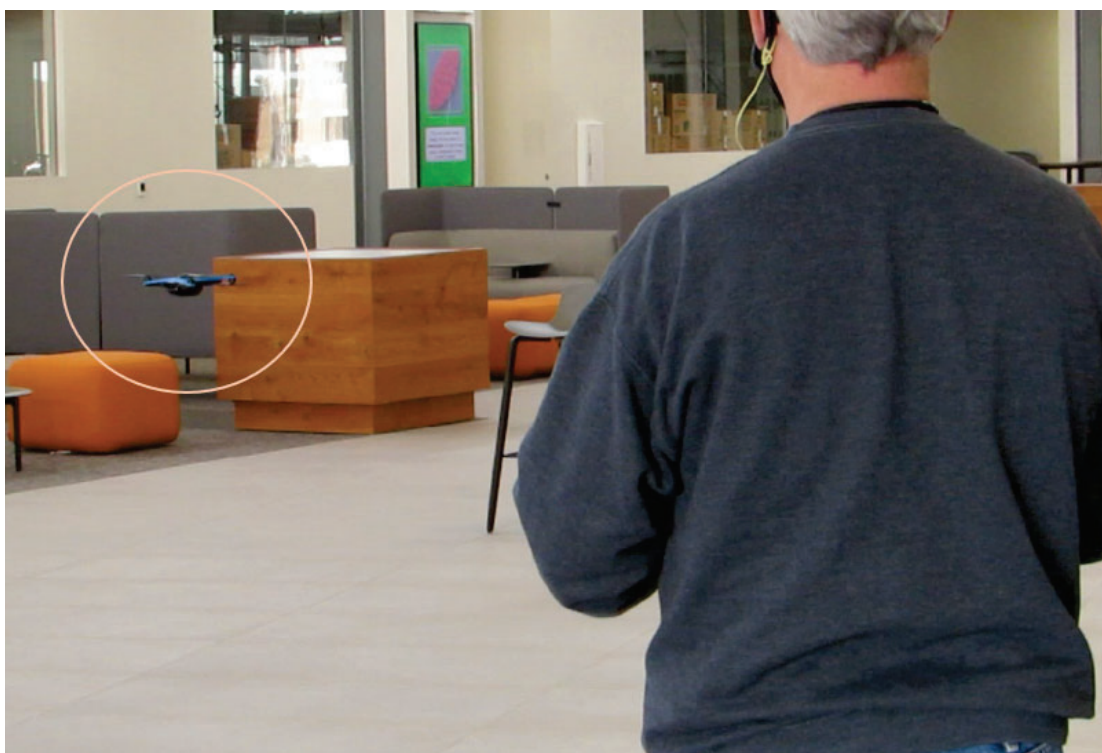
Figure E- 8. A small "Skydio S2" drone with a gimbaled 4K HD camera collects video imagery of a new PNNL building interior
