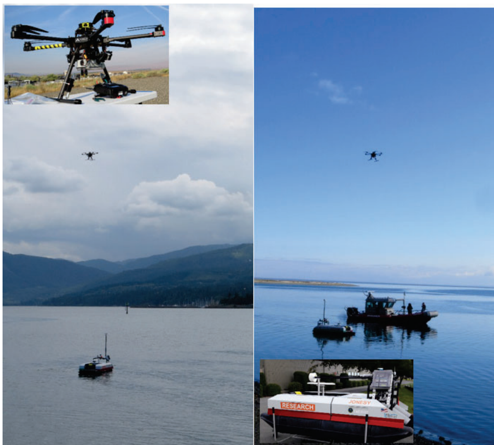
Figure E- 5. PNNL Operates surface and underwater autonomous systems at the PNNL Marine Science Laboratory located on the shore of Sequim Bay, WA. The images show one of our “X6” hexacopters interacting with an Unmanned Surface Vehicle (left) and the manned vessel (right) during a demonstration of autonomous collaborative behavior and communications capabilities. Inset images show the multirotor “X-6” UAS and the Autonomous Surface Vehicle.
