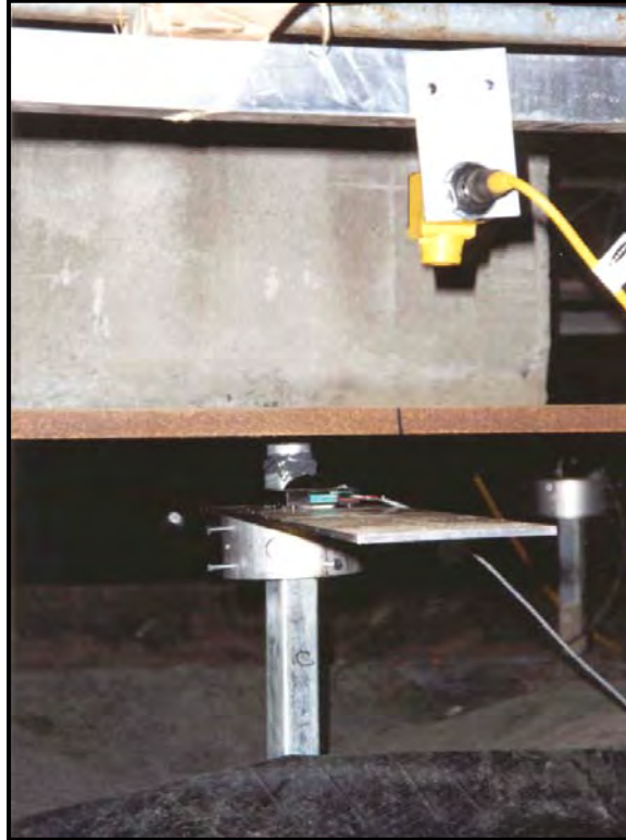
Figure 3.17 Support System for OMNI-BEAM™
