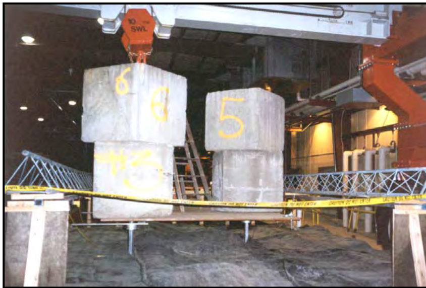
Figure 3.26 Loading Piers with Six Concrete Blocks
