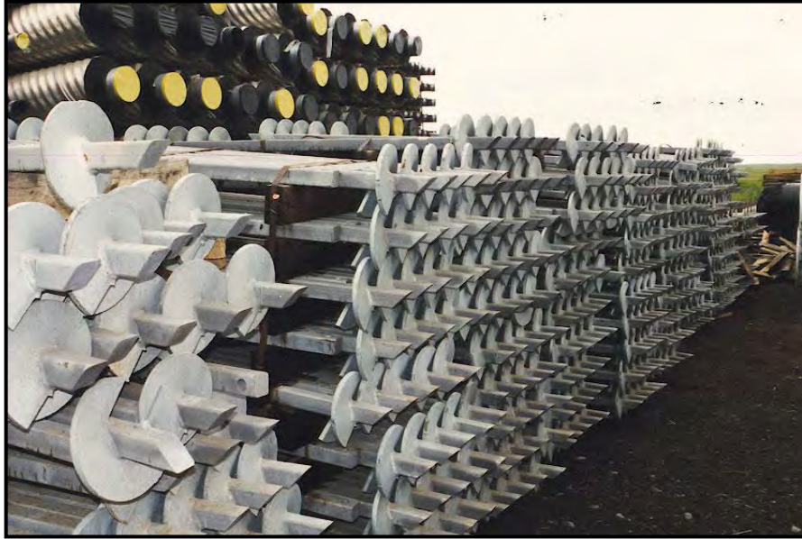
Figure 1.5 Helical Pier Stockpile in St. Michael, Alaska
