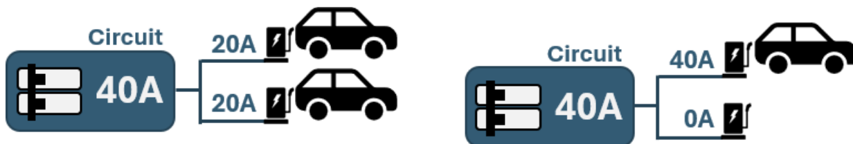
Figure 15. Circuit sharing is a strategy to share loads between EV chargers. This image shows a 2:1 ratio where each charger receives 20 amps from the same 40-amp circuit (Source: Courtesy of TRC).
