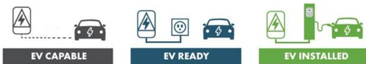
Figure 6. Building codes and standards reference three categories of electric vehicle infrastructure: EV-Capable, EV-Ready, and EV-Installed (Source: Blink Charging Co., modified by TRC).
