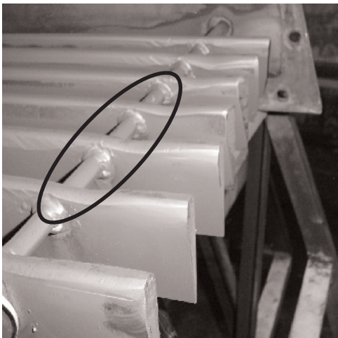
Figure 6 - No protective cladding on the flow element
