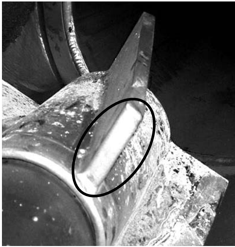
Figure 5 - Conforma Clad infiltration brazed tungsten carbide spreader shows no visible wear
