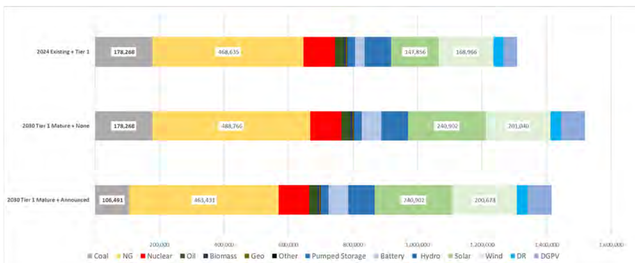
Figure A.9. Comparison of 2030 generation stacks for the various scenarios.
