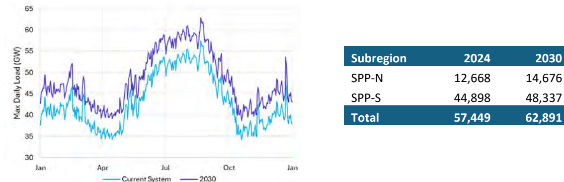
Figure 20. SPP Max Daily Load in the Current System versus 2030
