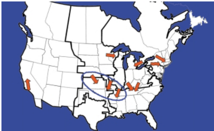
Figure 7-2 Current Electric Power Bottlenecks
