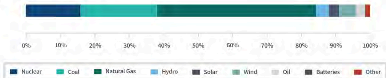
Figure 2-21: PJM Capacity Mix
