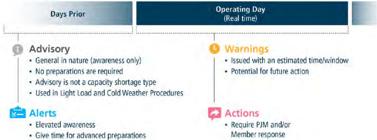
Figure 5. Emergency Procedure Levels
