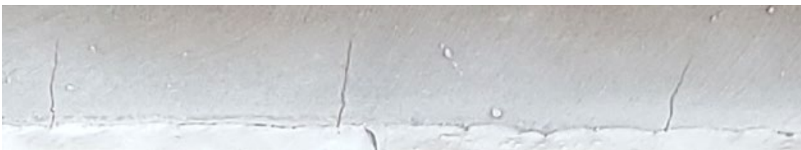
Figure 13. Magnified image of cracks in tri-span bolster
