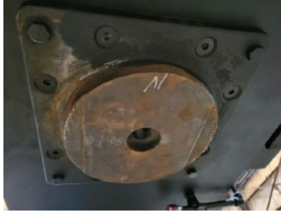
Figure 14. 12-bolt centerplate mounted to replacement Atlas tri-span bolster
