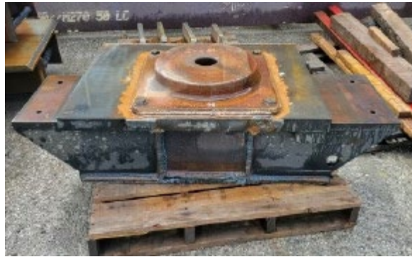
Figure 16. Tri-span section sent for NDE testing
