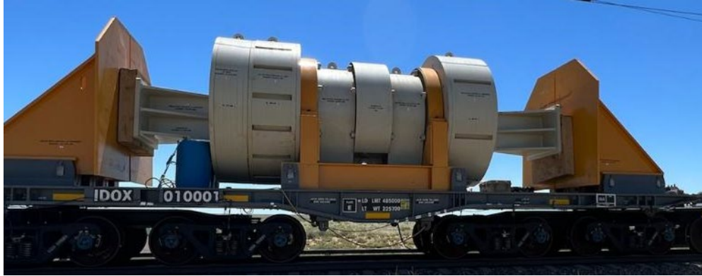
Figure 17. Dunnage problem: block on right side has slipped downward
