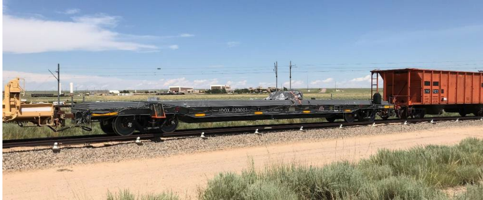
Figure 6. Buffer railcar IDOX 020001 during static testing
