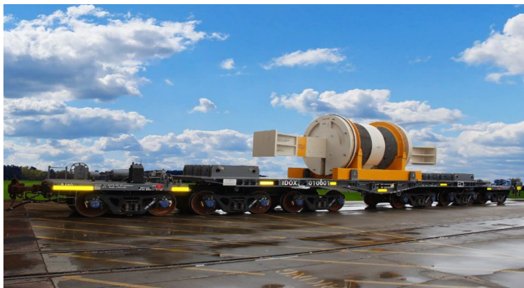
Figure 2. IDOX 010001 during testing with minimum test load
