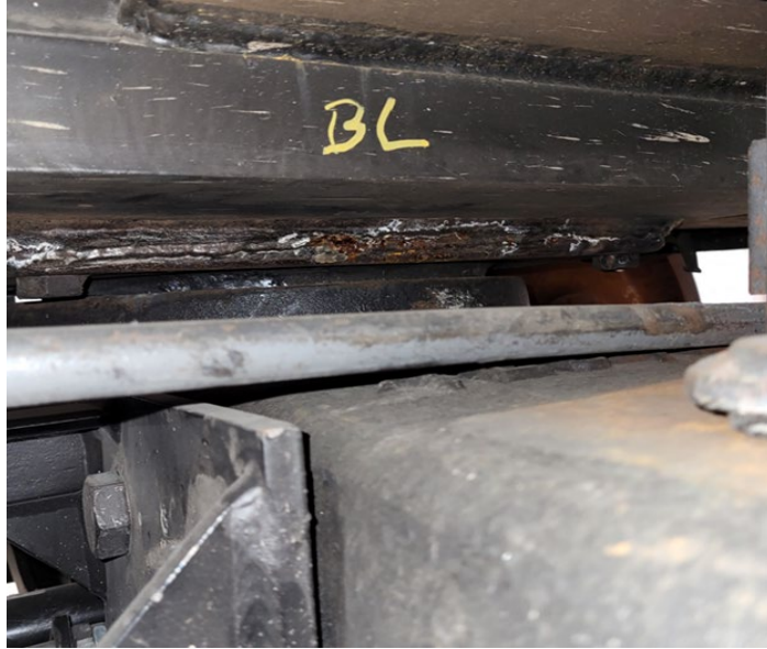
Figure 9. Atlas Railcar – Crack is on Left Side of Centerplate, B-Truck
