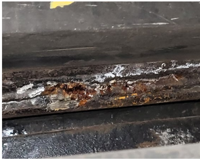
Figure 10. Atlas Railcar – Close-up of Crack on Left Side of Centerplate, B-Truck
