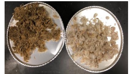
Deacetylated corn stover before and after ozonolysis
