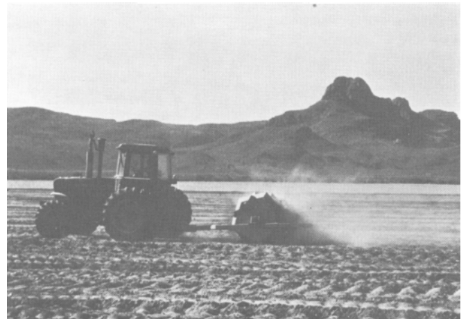
Figure 5. – Imprinter seeding a 243-ha desertified floodplain near Cortaro, Arizona in November, 1987. Imprinting and seeding the floodplains as well as the upper parts of the watershed can prevent destructive flash flooding (and associated erosion and sedimentation) of the river channel.
