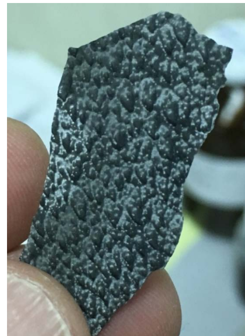
Sample of scale from March 2017 test of IWTU.
