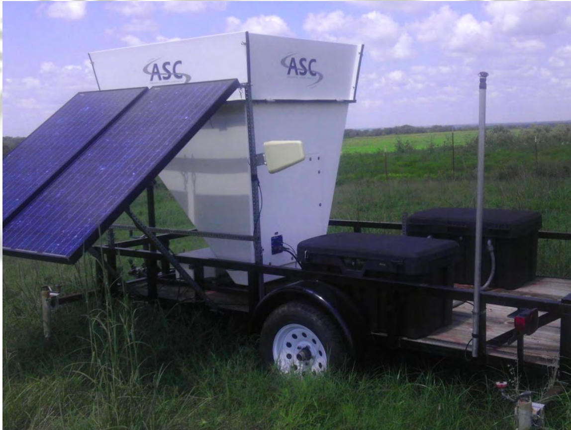
ASC SODAR Unit Solar Panel and Battery Pack
