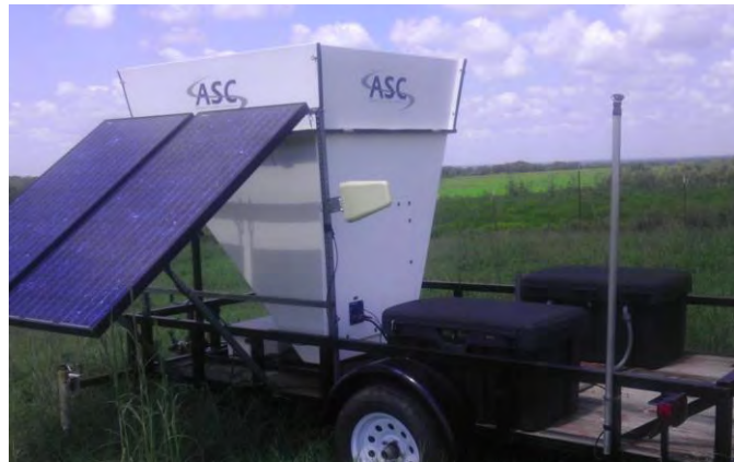
Figure 1. ASC SODAR Unit Solar Panel and Battery Pack
