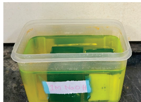
Figure 10: PTFE/EPDM-wrapped aging configuration showing the protected grout and exposed epoxy surface (left) and the wrapped specimens immersed in 1 M NaOH solution during the seven-day leakage trial (right)
