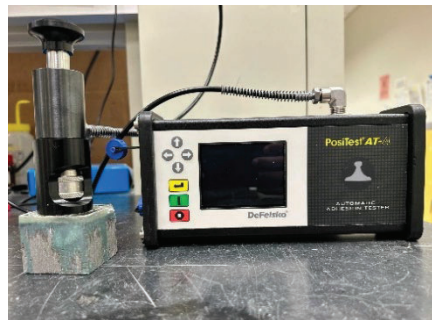
Figure 4: Pull-off adhesion test showing the test principle (left) and the portable pull-off adhesion tester used in this study (right)
