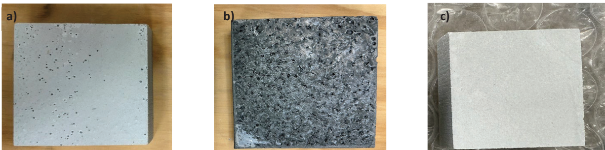
Figure 2: Representative as-cast grout specimens before surface characterization and epoxy application: (a) Grout A, (b) Grout X, and (c) Grout BC
