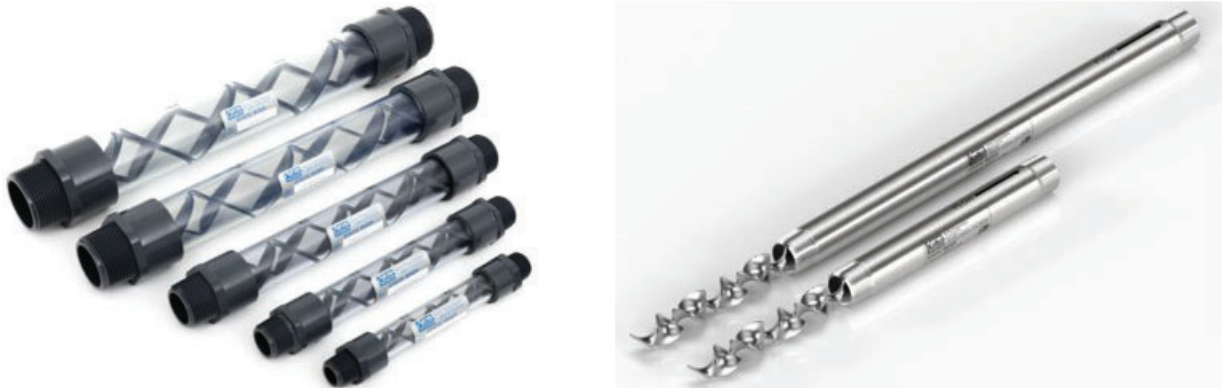
Figure 15: Examples of in line mixers. Clear PVC piping with baffles visible inside on the left. Stainless steel piping with high viscosity baffles partially removed and shown on the right for high viscosity liquids like two part epoxies.
