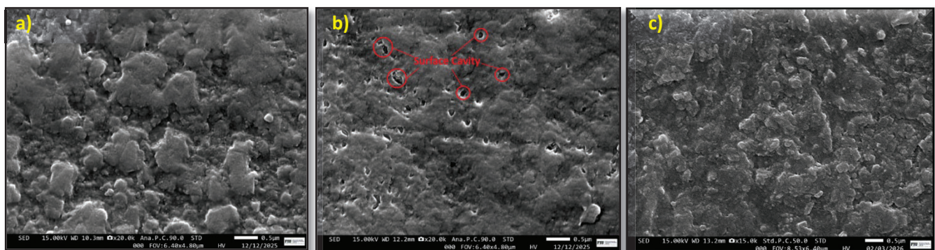
Figure 8: SEM images showing the near-surface morphology of (a) Grout A, (b) Grout X, and (c) Grout BC
