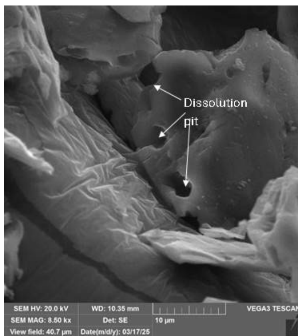
Figure 2.14. Scanning electron microscopy (SEM) image showing dissolution pits on reacted gibbsite surfaces
