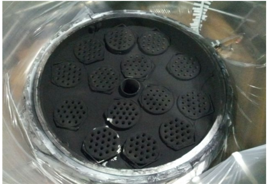
Off-Gas Filter Photo—Top of Filter Bundle Tubesheet, Post-Event
