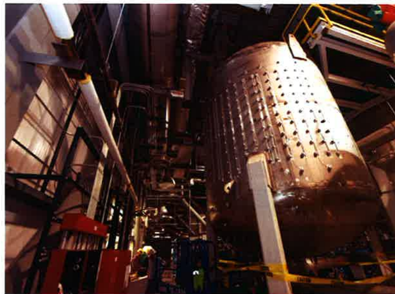
One of two mercury adsorber vessels in the off-gas treatment system
