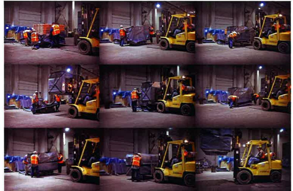
AMWTP employees place a box of primary waste in a DOT shipping bag to preserve its integrity during shipping. This box of waste will be sent to Energy Solutions, Inc. for permanent disposal.
