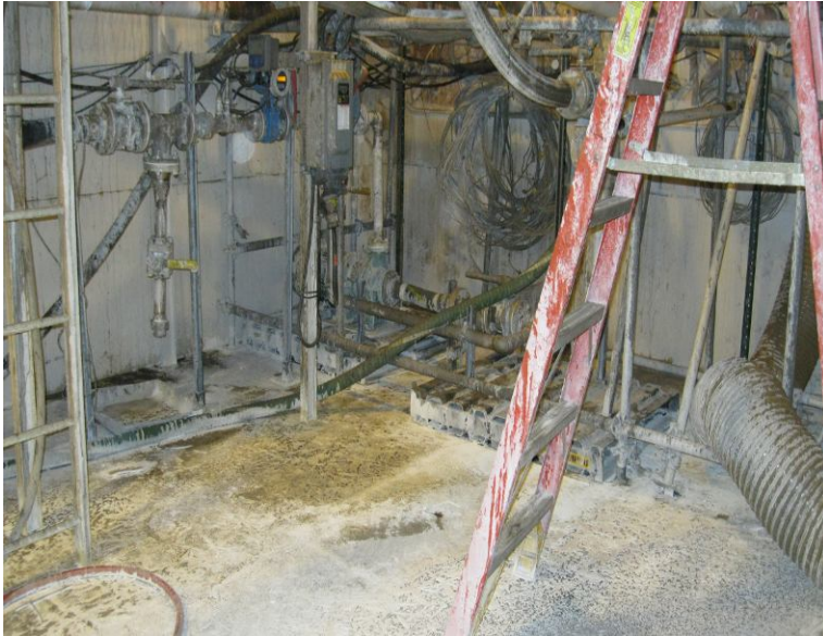
MFC-766 caustic solids before pressure washing
