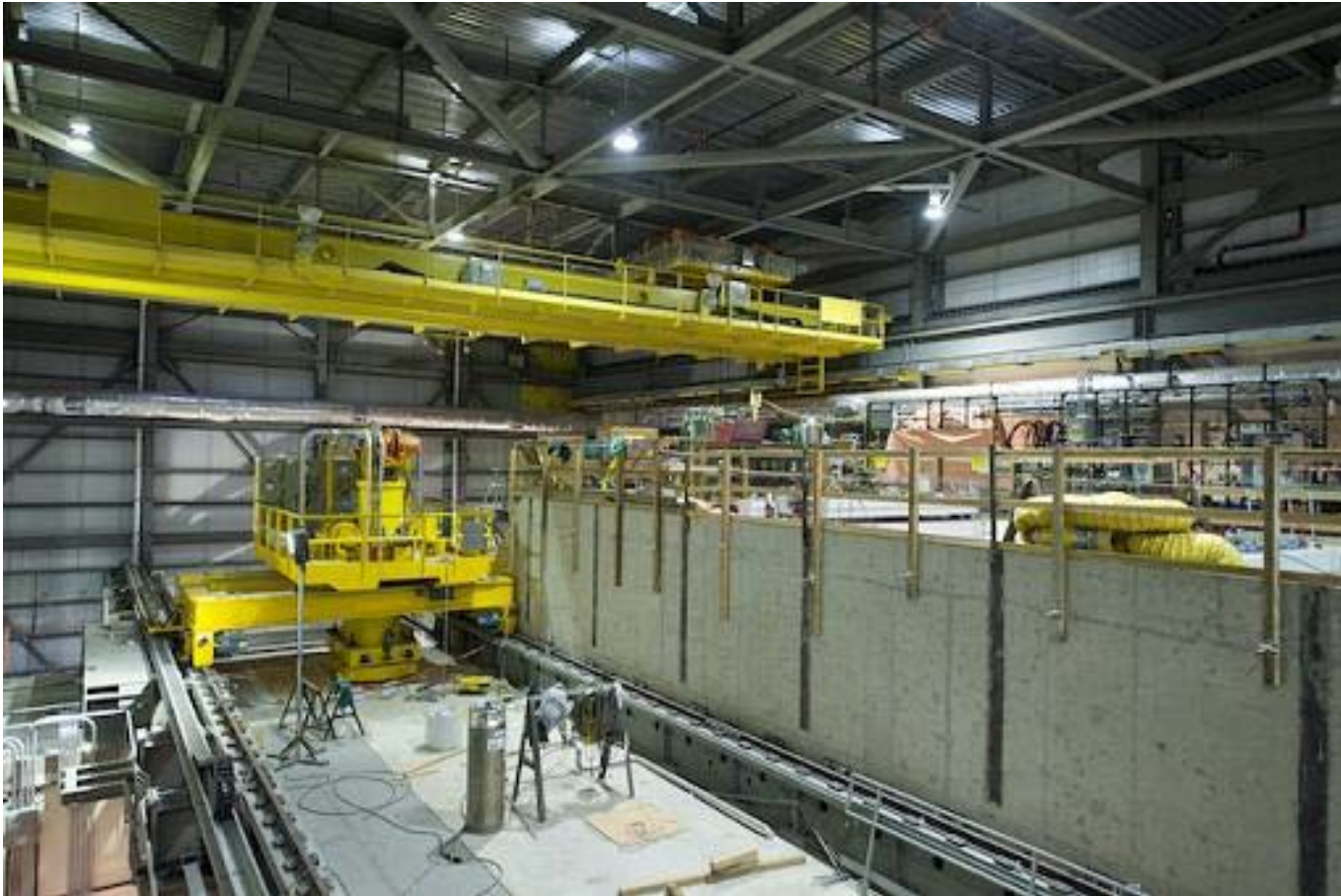
Transfer Bell Crane and Maintenance Crane
