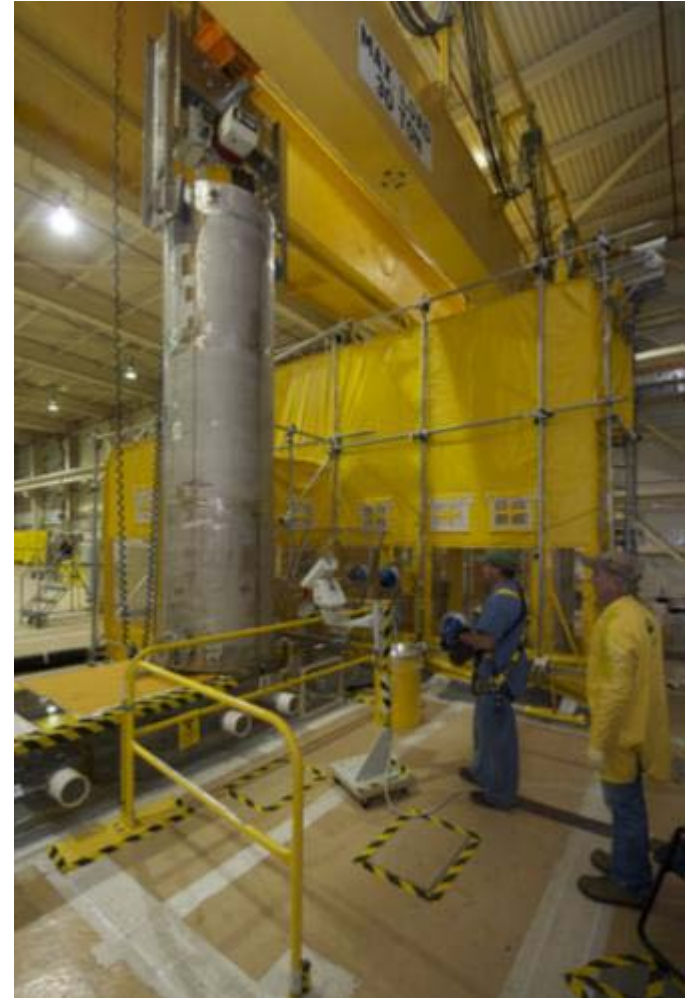
Repackaging an RH-TRU liner in the FDP
