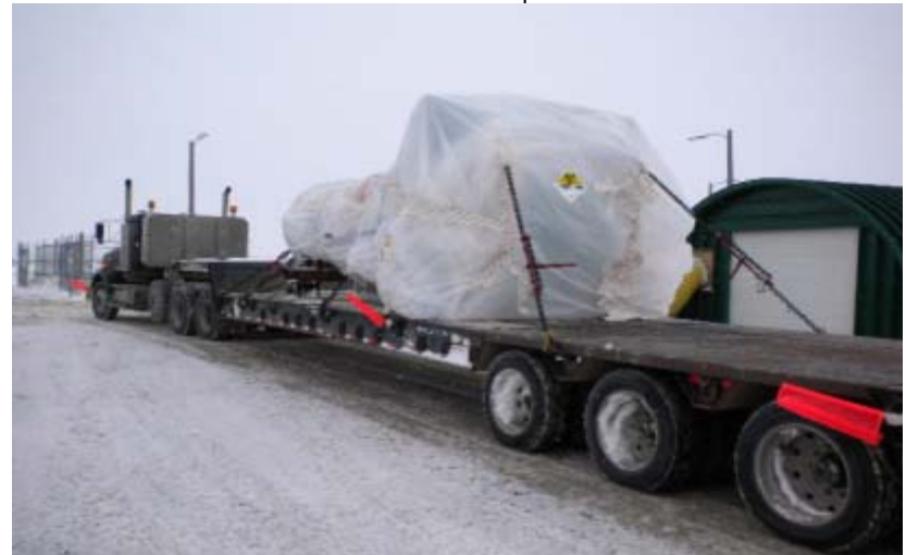
MTR Reactor vessel transportation to ICDF
