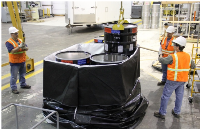
Above: Loading MLLW product drums in macro-encapsulation bag
