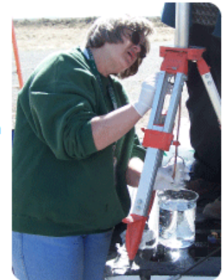
USGS technician sampling for dissolved gases, photo by USGS
