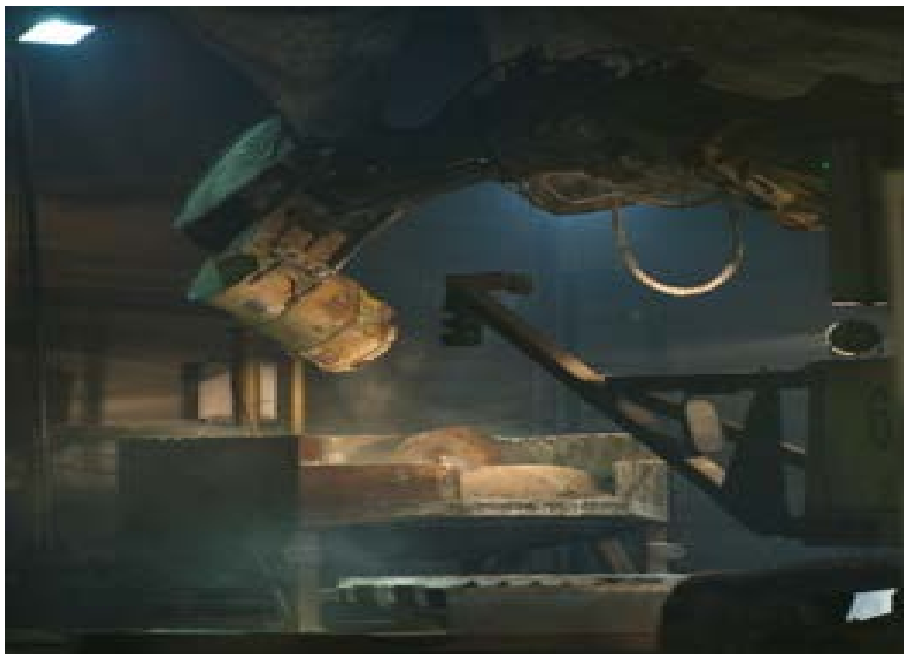
Above: Excavator empties sludge into trays in ARP V.
