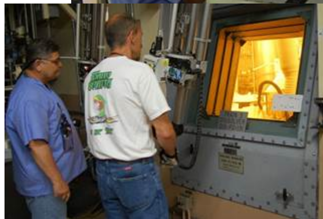
Left and Above: Repackaging RH- TRU waste in hot cells.
