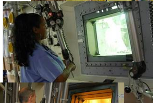
Left and Above: Repackaging RH- TRU waste in hot cells.
