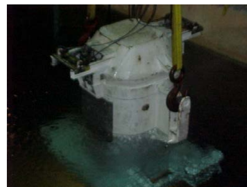
High-Load Charger used to transfer ATR SNF
