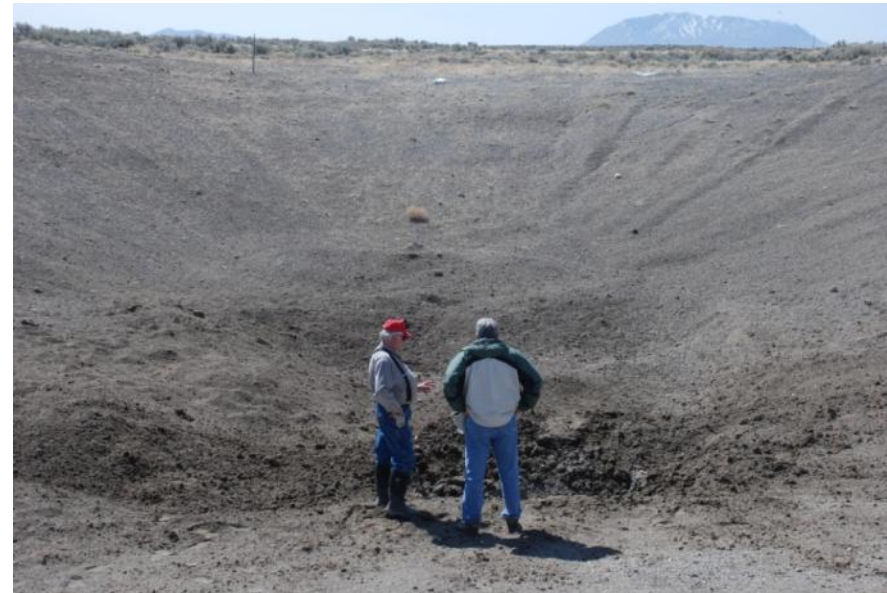
MDA crater following propellant detonation
