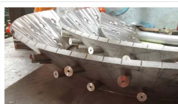
Upper cone and nozzles
