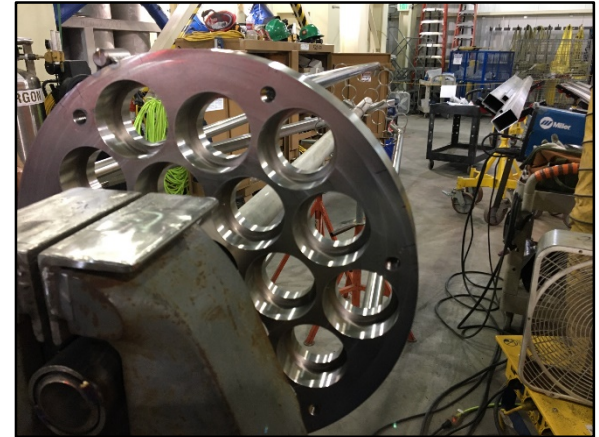
Filter bundle being fabricated
