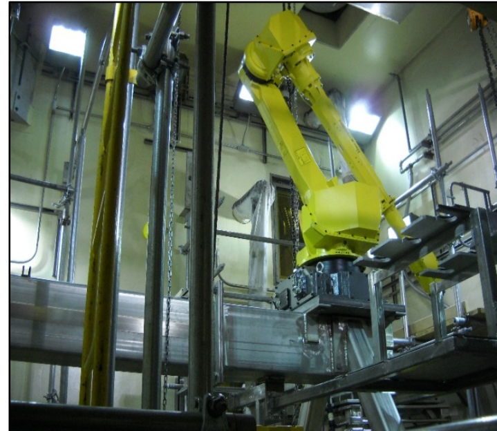
Robotic arm installed in Can Fill Cell 1
