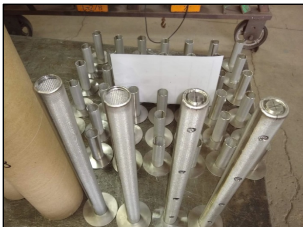
Truncated fuses in background Perforated and drilled out fuses in foreground
