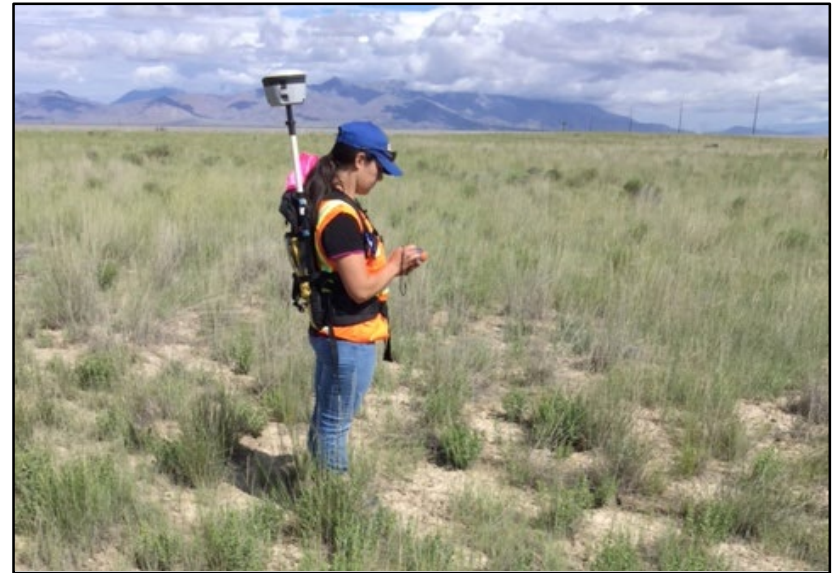
Routine CERCLA field inspections at CFA landfill. Inspections include evaluation of vegetative cover and looking for signs of erosion, subsidence or animal intrusion.
