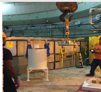
30 gallon shielded container for RH TRU waste
