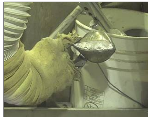
Bulk sodium found inside a pipe during treatment of RH waste
