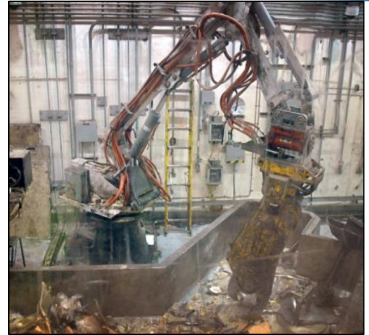
BROKK robotic arm for sizing waste
