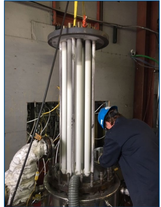
PGF Refractron ceramic filter bundle at Hazen
